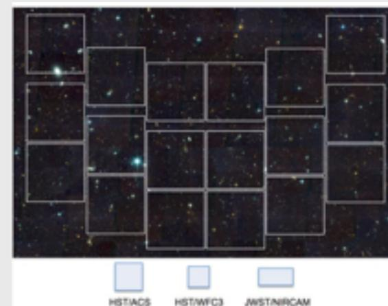
WFIRST/WFI FOV vs other instruments on HST and JWST. Each of the 18 individual white boxes represents one detector in the WFI FOV.
