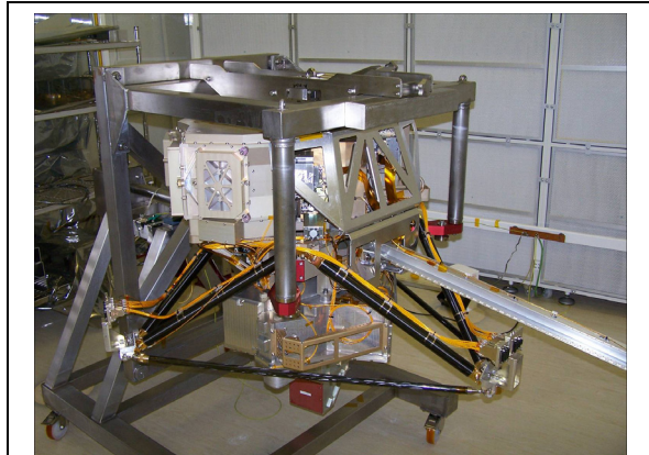
Figure 6. MIRI verification model going into thermal vacuum testing. Credit: European MIRI consortium; used with permission.
