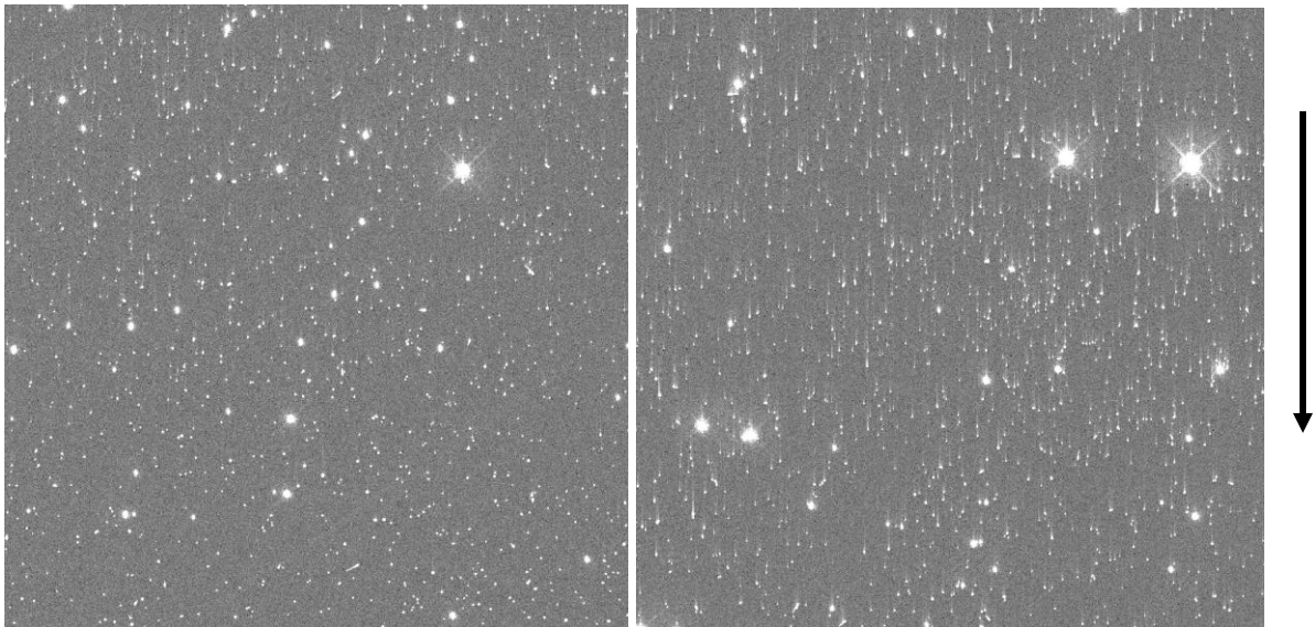
Figure 1. At left, a 1000x1000 pixel image subsection closest to the amplifier which in this case is at lower left. At right, a 1000x1000 pixel image subsection furthest from the amplifier. Neither exposure has had a post-flash applied; the sky background was \sim 0 e-/pix. The readout direction is marked with an arrow.
