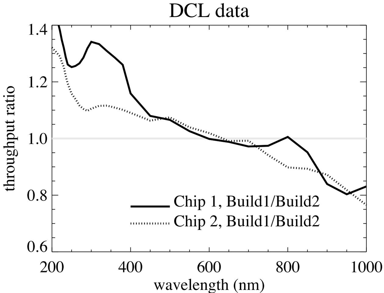
Figure 3: The ratio of throughputs for Build 1 and Build 2, on a chip by chip basis, based upon DCL data for the detector QEs and Ball Aerospace data for the optics. This is an appropriate comparison, because Chip 2 is the better performer in the UV in both datasets.
