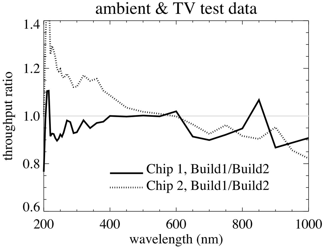
Figure 4: The ratio of throughputs for Build 1 and Build 2, on a chip by chip basis, based upon the measurements in the 2004 thermal vacuum tests (Build 1) and 2007 ambient tests (build 2).
