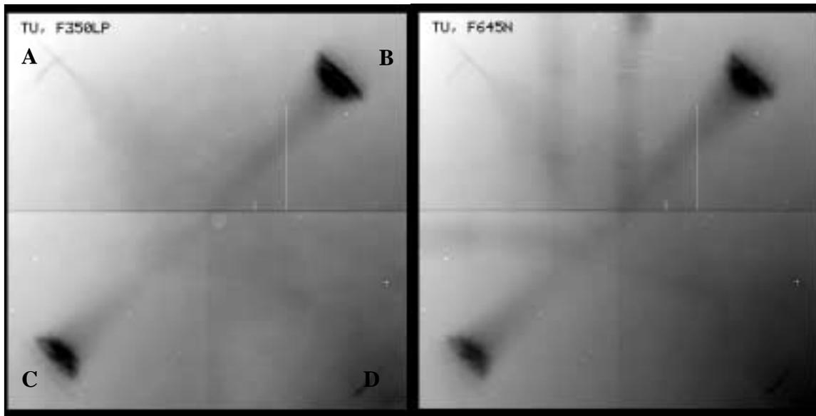
**Figure 1:** At left is a typical UVIS calsystem flatfield with the tungsten lamp, displayed with a hard inverted stretch to highlight features; quadrants are marked. At right is a tungsten calsystem flatfield through the f645n filter, showing additional vertical and horizontal reflections. Tungsten flatfields using other filters are shown in Appendix B.
