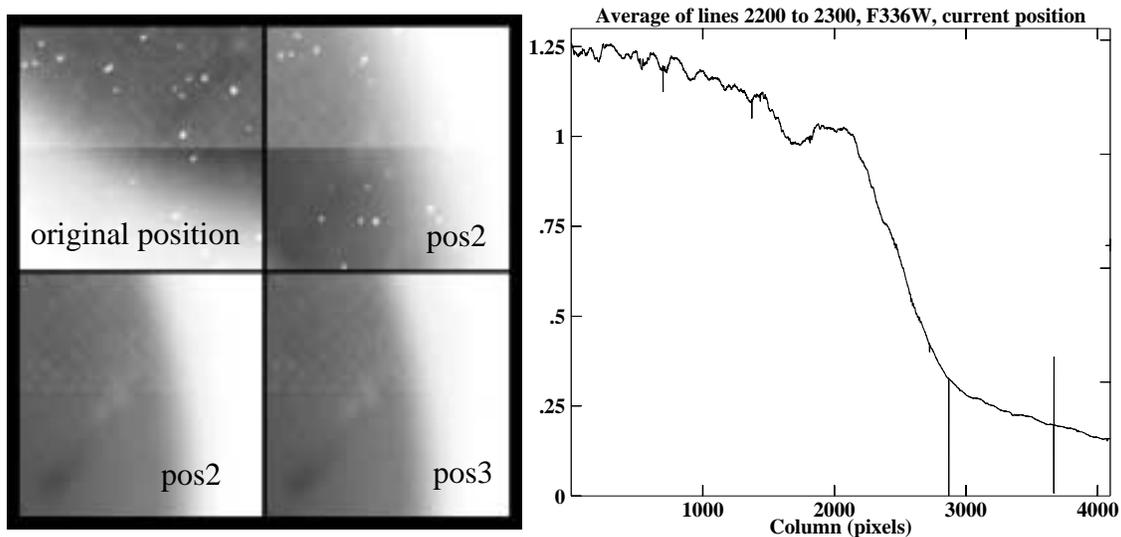
**Figure 3:** Mosaic of four full-frame D2 calsystem flatfields, shown in an inverted stretch. The two upper images are F225W: left is from May 2004 with the D2 lamp in its original position, right is the result of the first realignment. Bottom images are F336W: left is after the first realignment, right is after the second realignment (the current position). The plot at right shows a 100-row wide cut through the current position flatfield.
