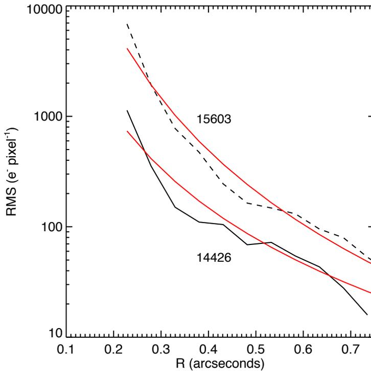
**Figure 4: Measure of the residual speckle noise seen over the two coronagraphic programs 15603 (dashed line) and 14426 (solid line). The red curve denotes the best fit power-law relation fit for each program. The scale of the noise is related to a power-law curve and scaled by the peak brightness of the PSF, estimated to be  $2.08 \times 10^8$  e<sup>-</sup> pixel<sup>-1</sup> in a 1s exposure.**
