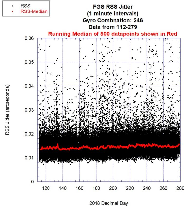
**Figure 3: Measure of RSS jitter during the time period that the 2,4,6 gyro combination was active. The red curve denotes a running 500 point median which roughly corresponds to a 24-hour period of time.**
