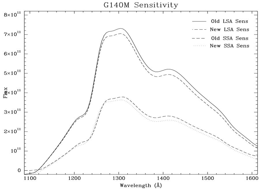
**Figure 6:** The previous sensitivity functions are plotted with the corrected curves, illustrating the extent of the change required to match the G140M data with the reference spectrum of  $\mu$  Col.
