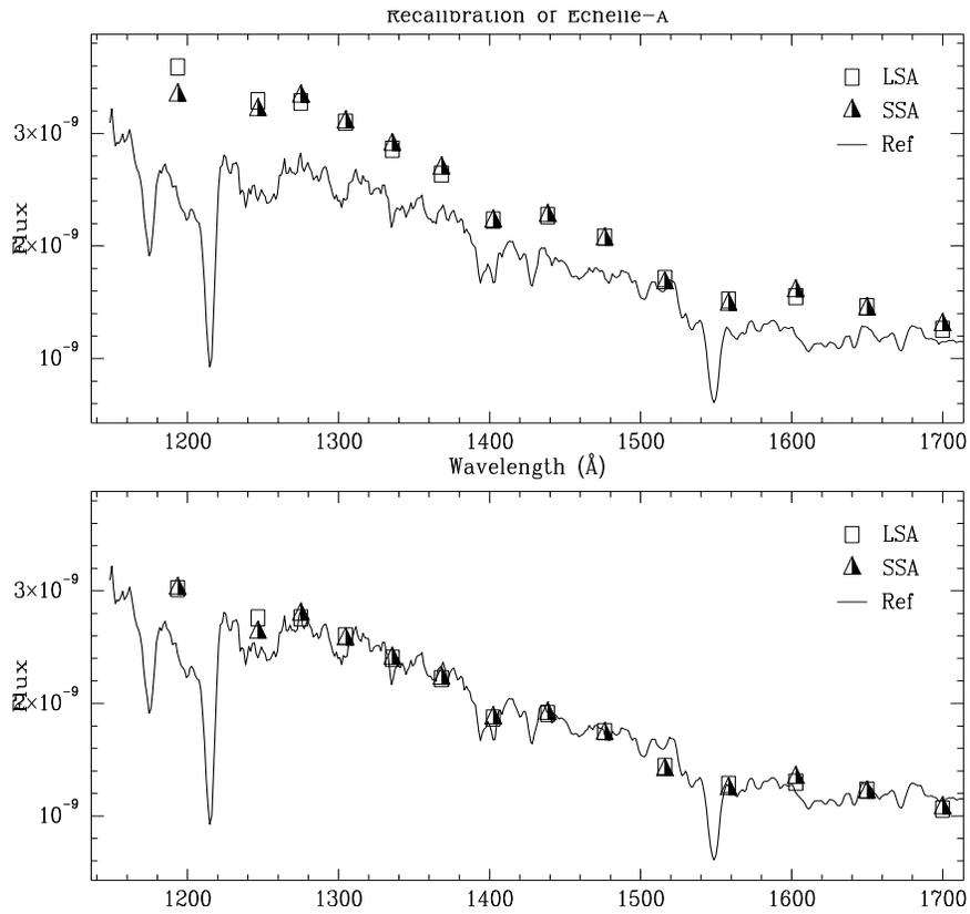
**Figure 2:** The reference flux for  $\mu$  Col is plotted with the calculated values from Echelle-A. *a)* Both LSA and SSA show an excess flux of  $\sim 19\%$  using the old sensitivity file. *b)* Measured and reference flux values agree once a constant factor is applied.
