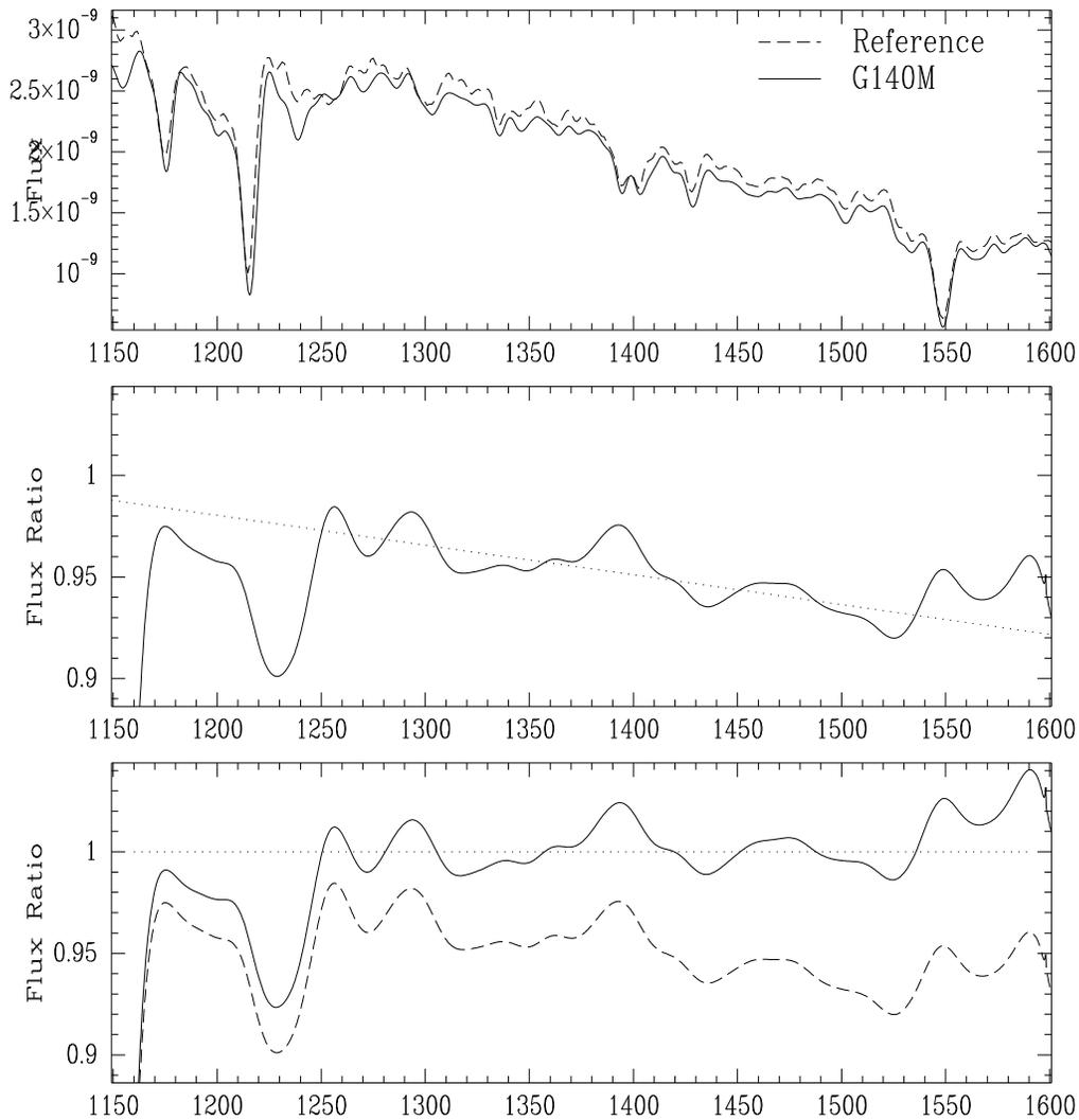
**Figure 4:** *a)* The reference IUE spectrum for  $\mu$  Col is plotted with the merged G140M data using the most current reference files. *b)* The ratio of G140M to the reference spectrum is fit with a linear function for use in correcting the sensitivity. *c)* Applying the linear correction to the current sensitivity function improves the ratio dramatically.
