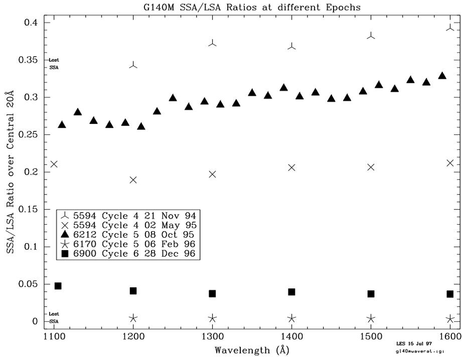
**Figure 5:** The SSA/LSA ratio is plotted for each of the G140M calibration proposals. The ratio is determined for each file, using no flux correction, and using the central 10 Å of each dataset.
