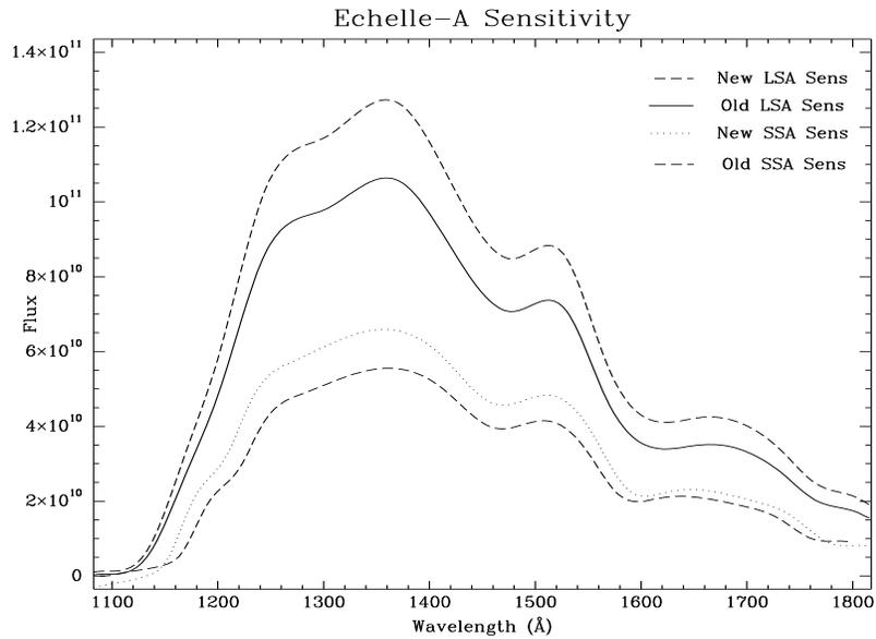
**Figure 3:** The sensitivity function (e5v0936nz.r3h) for the LSA and the SSA is plotted with the new sensitivity file with the appropriate corrections.
