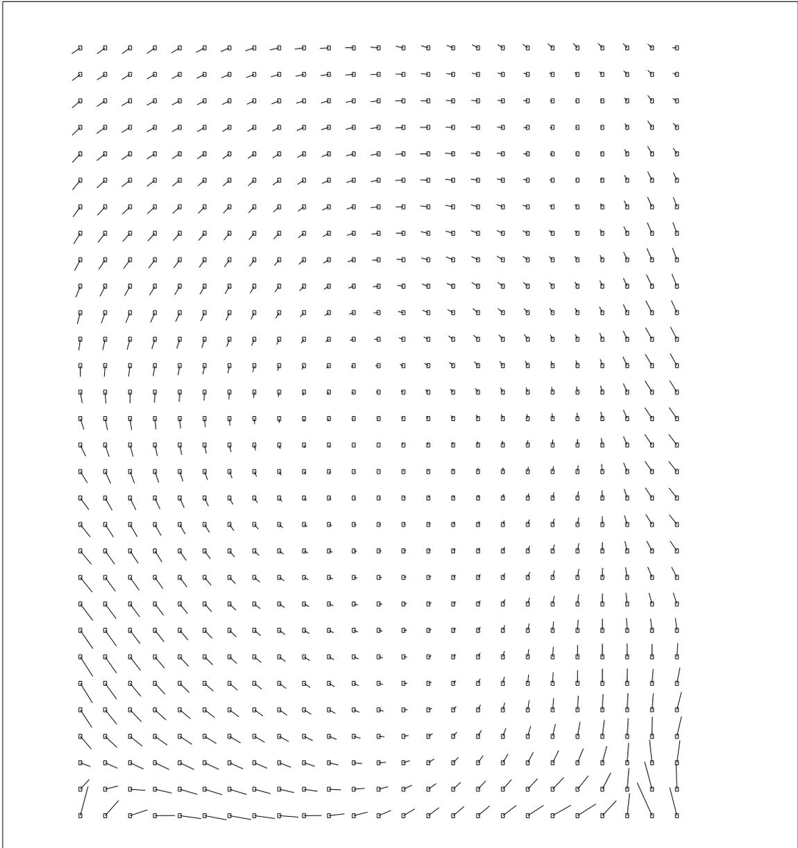
**Figure 7.** The difference between the new distortion model vectors and the distortion model vectors (ISR FOC-086) for the 512×512 format shown magnified on a grid with a spacing of 16 pixels. Because of the large distortion effects near the edges, the distortion differences are not shown near the edges.
