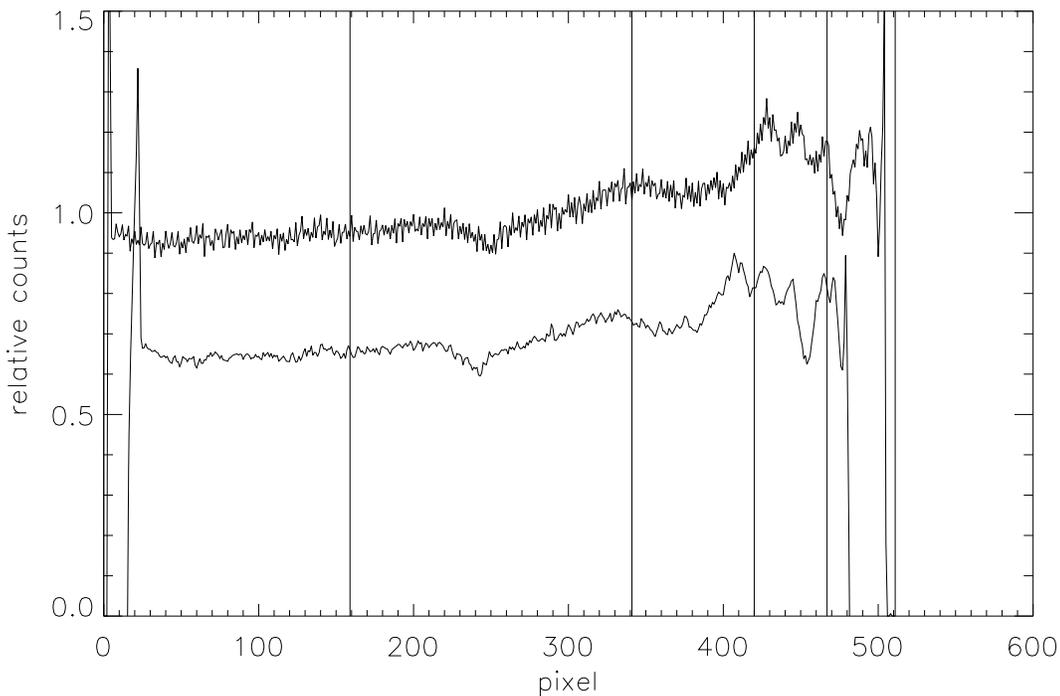
**Figure 11.** The average of rows 200 through 500 of the 512×512 LED flat field. The top curve shows the average for the raw image while the lower curve shows the average for the geometrically corrected image. Both curves have been normalized by the average value in the averaged region. The lower curve has been offset by 0.4 to clearly separate it from the upper curve. The vertical lines show the location of the x knots which are valid only for raw image coordinates.
