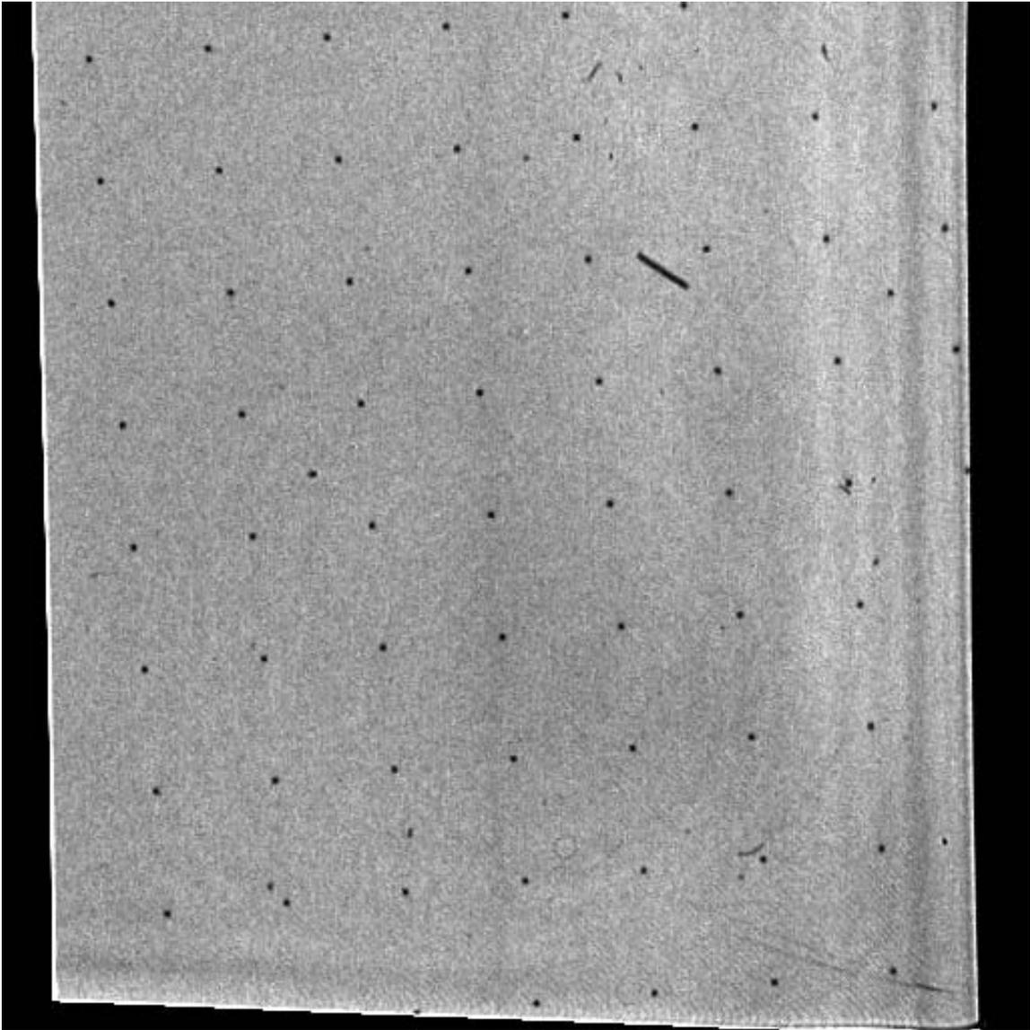
**Figure 10.** A 512x512 LED flat field that has been geometrically corrected using the latest geometric correction model. Note the photometric variations near the beginning of the scan line (the right hand edge) that appear as vertical features have not been removed as a result of the geometric correction.
