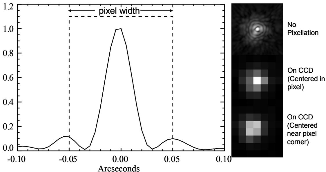
Figure 4. (Left) Cross-section through a computed HST PSF at  $\lambda = 336$  nm. The width of a WFPC2 WF pixel ( $0.1''$ ) is shown. (Right) On top, the computed 336 nm HST PSF prior to pixellation. Below it is the PSF centered at the middle of a pixel and in the corner, integrated over the WFPC2 WF pixel area, shown at the same spatial scale.
