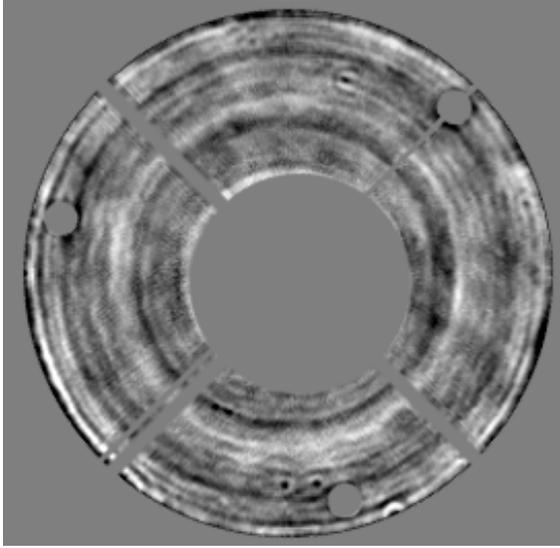
Figure 2. Map of the combined primary and secondary mirror surface errors left from polishing obtained using phase retrieval on highly defocused star images. Shown between  $\pm 30$  nm surface error. The HST and WFPC2 obscuration patterns are superposed.
