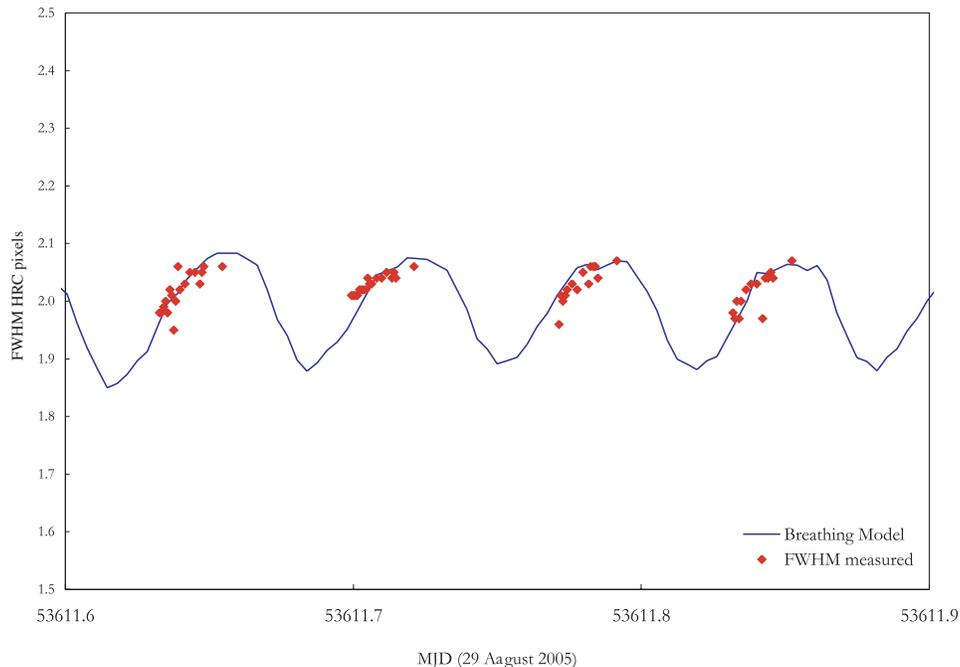
**Figure 1.** PSF Full-Width at Half-Maximum (FWHM) measurements in the ACS/HRC as part of the Two-Gyro Servicing Mission Orbital Verification (TGSMOV) testing. The broadening of the observed PSF over time is consistent with variations expected due to the “breathing” of the HST OTA during a typical orbit. The typical change in the PSF FWHM in this figure is  $\sim 0.1$  pixels.
