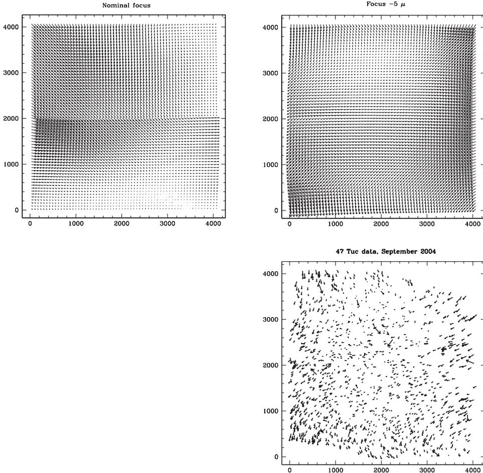
**Figure 2.** PSF ellipticities in the ACS/WFC measured from Tiny Tim PSF models. At top-left: ellipticities measured from models at nominal focus. At top-right: ellipticities measured from models at  $\sim -5\mu\text{m}$  of SM despace. At bottom-right: PSF ellipticities of stellar sources in 47 *Tuc* observed in the ACS/WFC with *F814W* while *HST* was known to be in a negative focus state of  $\sim -5\mu\text{m}$
