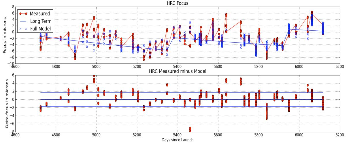
Figure 2. A history of the HRC focus. The upper plot shows the measured values (Lallo et al. 2010), the secular model and the full composite model. The secular model includes steps corresponding to the occasional adjustments made to the secondary mirror position. The lower plot shows the difference between the measured and modeled values. The blue lines indicate the mean value and one standard deviation above and below the mean.
