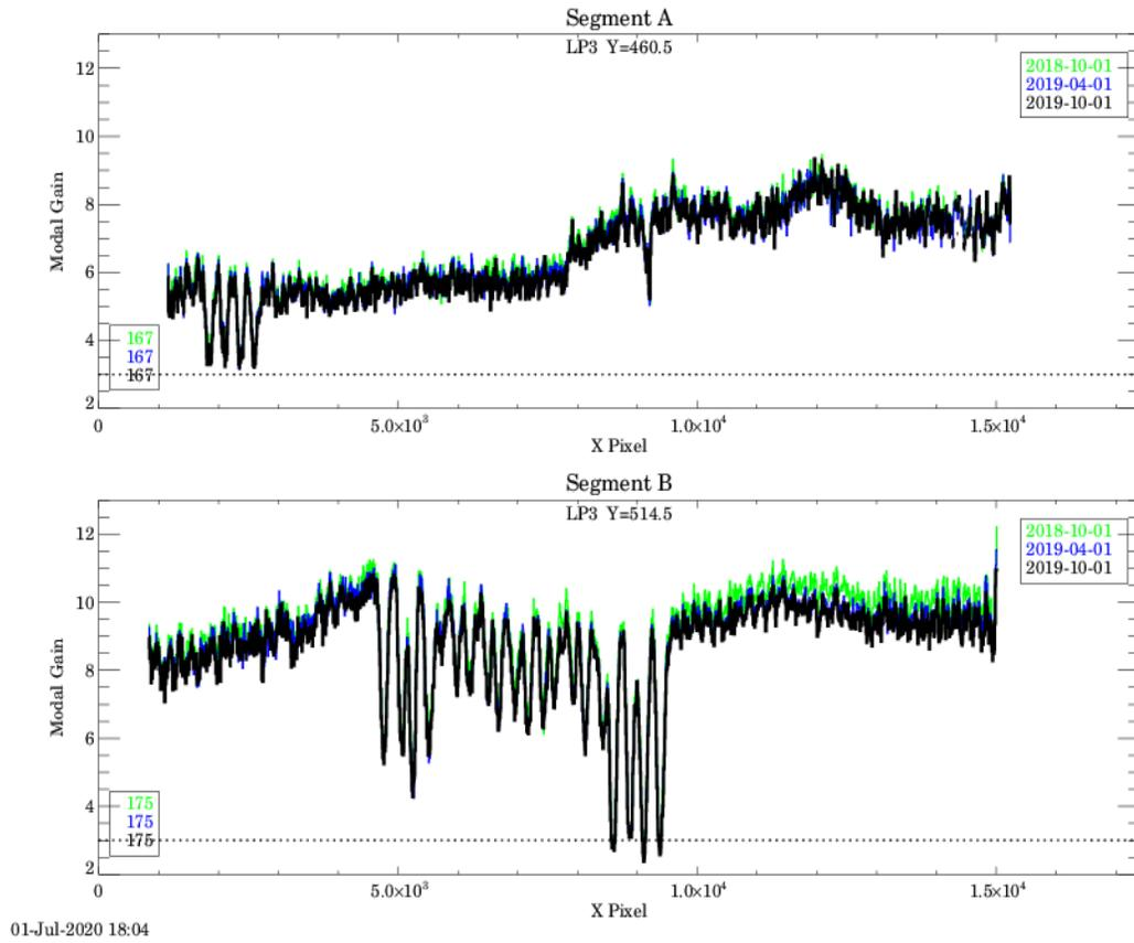
Figure 3. Modal gain as a function of X pixel at the center of the LP3 region of the detector using the LP3 G130M/1222 HV values of 167/175.
