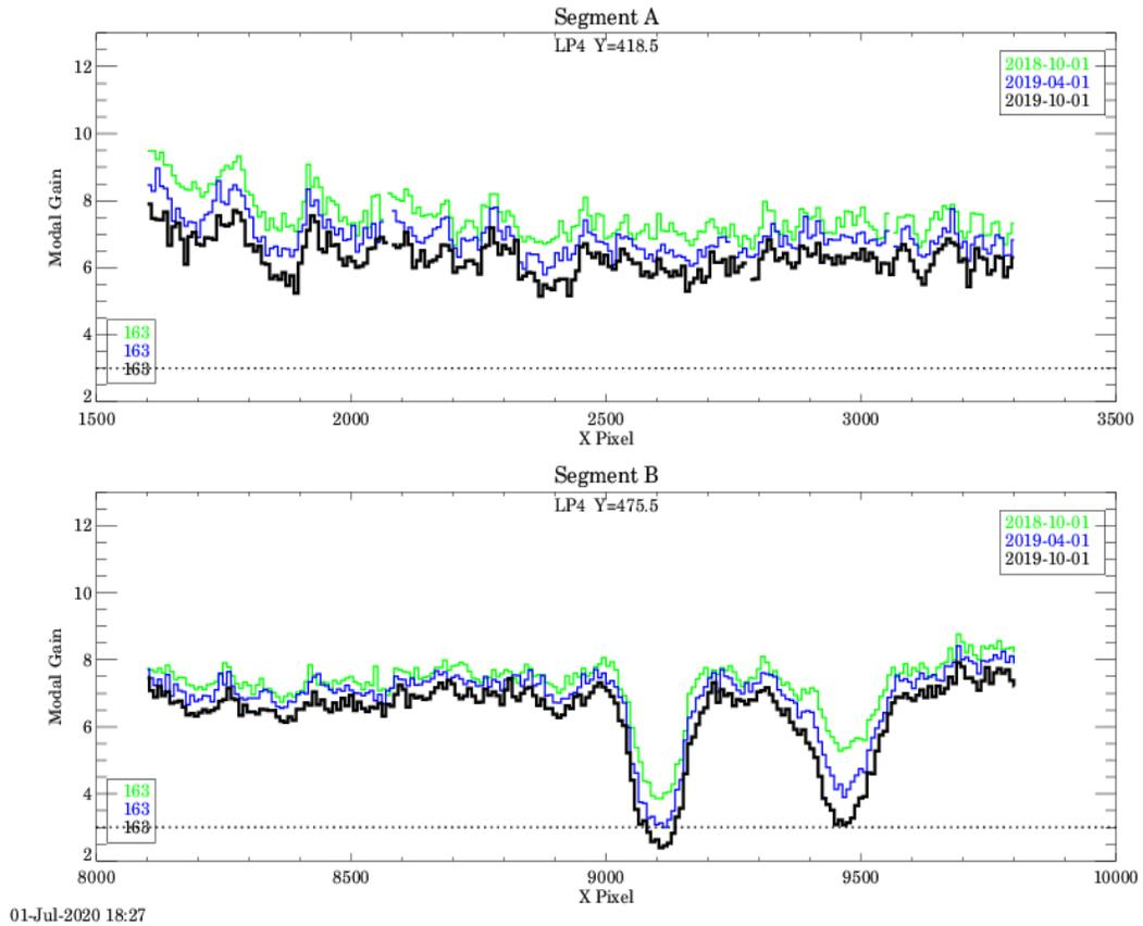
Figure 2. Zoomed in view of the data shown in Figure 1. This view highlights the significant drop in modal gain on Segment B at the positions corresponding to the Lyman- $\alpha$  lines from G130M/1291, FP-POS 3 and 4. These are the only FP-POS values that place Lyman- $\alpha$  on this segment at LP4. We allow the modal gain at these locations to drop below 3.
