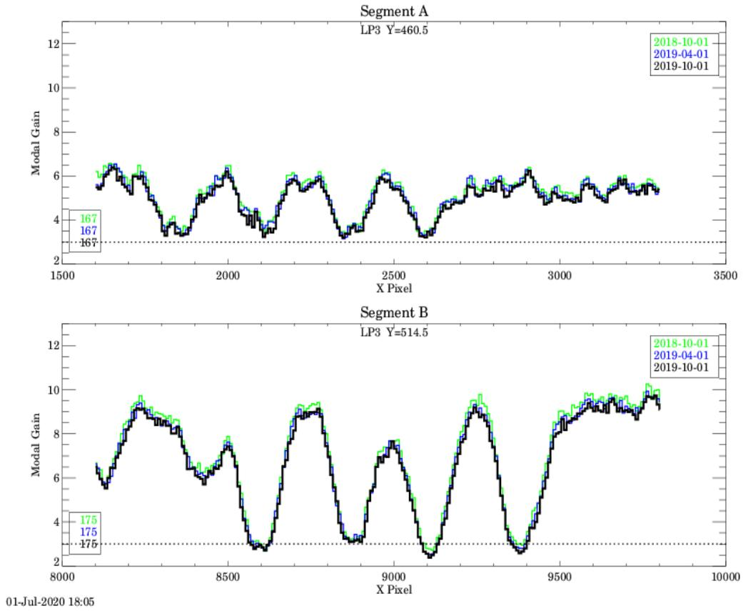
Figure 4. An expanded view of a portion of the modal gain plot shown in Figure 3. All four Lyman- $\alpha$  lines due to G130M/1291 at LP3 on Segment B have dropped to a modal gain of  $\sim 3$  at HV=175. On Segment A, the four Lyman- $\alpha$  impacted regions are approaching this value, but since the current HV is only 167, it can be raised before a loss of counts occurs.
