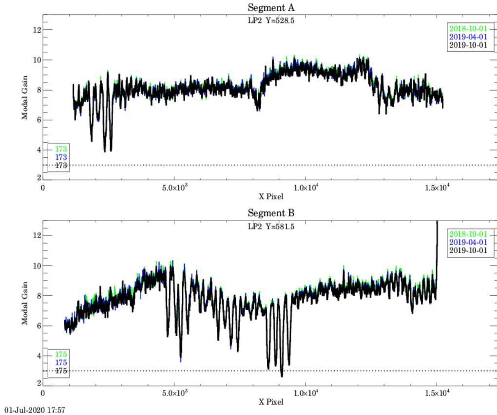
Figure 5. Modal gain as a function of X pixel at the center of the LP2 (Blue Mode) region of the detector using the Blue Modes HV values of 173/175. There was very little change during this cycle, which is not surprising since this mode is not used extensively. The deepest hole has a modal gain of  $\sim 3$ , where throughput losses are  $\sim 5\%$ .
