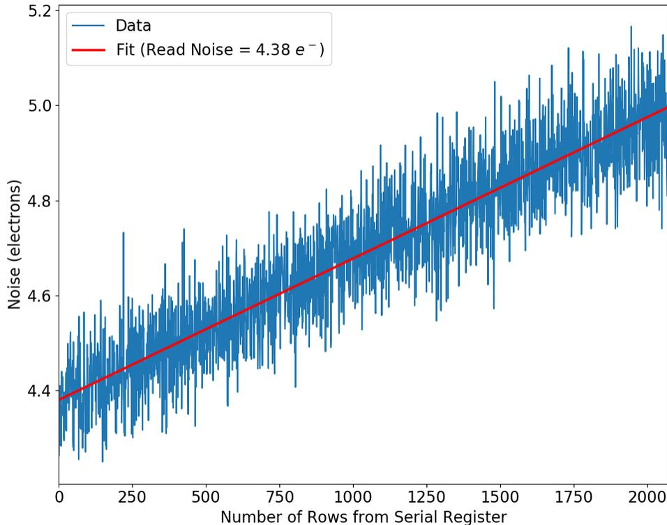
**Figure 1:** The fit to the noise as a function of row number (increasing away from the serial register) for readout amplifier A. The positive correlation between noise and row number is due to the presence of dark current accumulated during the readout of the WFC CCDs. Read noise values reported here and in calibration files are the intercepts of the fits at row 0.
