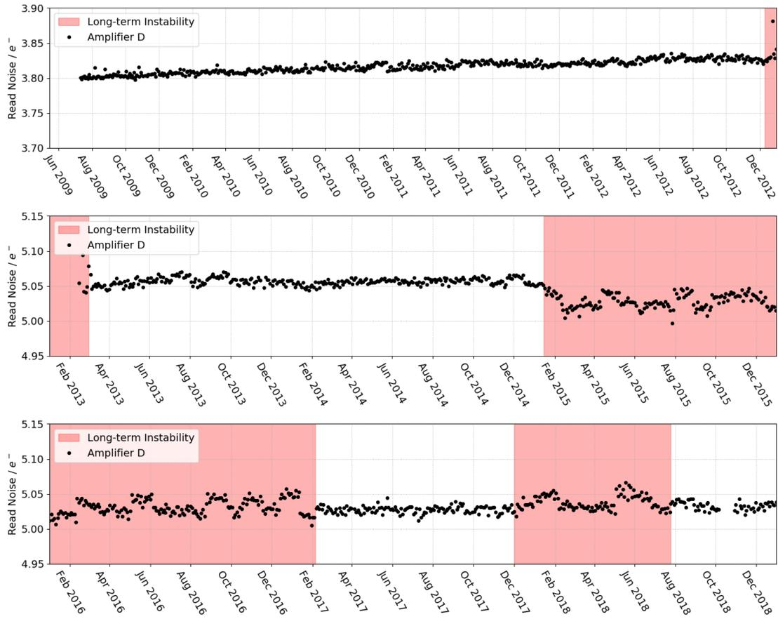
**Figure 4:** The same as in Figure 3, but for readout amplifier D. The y-axis limits in the top panel reflect read noise values before the anomaly in January 2013, while the middle and bottom panels have limits consistent with post-anomaly values. The scale of y-axis in all panels of Figures 3 and 4 is the same for comparison.
