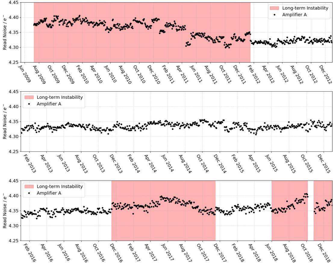
**Figure 3:** Expanded plot of the read noise as a function of time for readout amplifier A. The y-axis values on each panel are identical. Periods of markedly unstable behavior in the read noise have been shaded in red.
