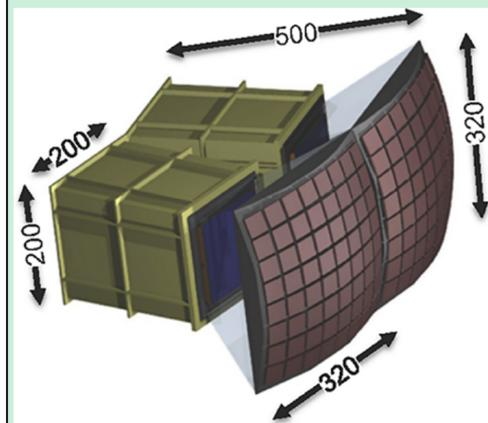
**Figure 1.** Two of four SBE-WFXT modules for localizing SBO events of CCSNe. Dimensions provided are in mm.
