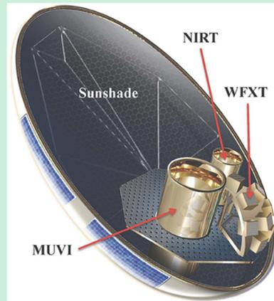
**Figure 2.** SBE S/C concept would not include a NIRT, fewer WFXT modules, and a smaller sunshade.
