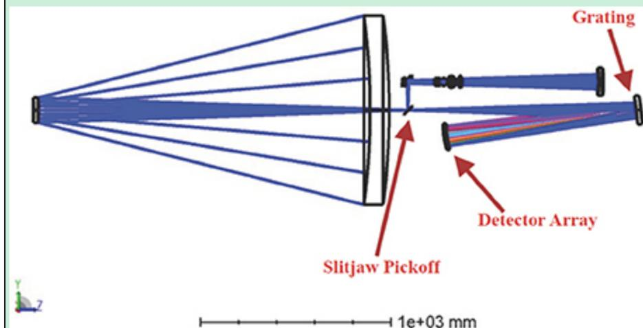
**Figure 3.** MUVI telescope, spectrograph, and imager design. This design offers high throughput while maintaining low-resolution spectroscopy and approximately arcsecond-level imaging for SN localization, galactic characterization, and light curve follow-up.
