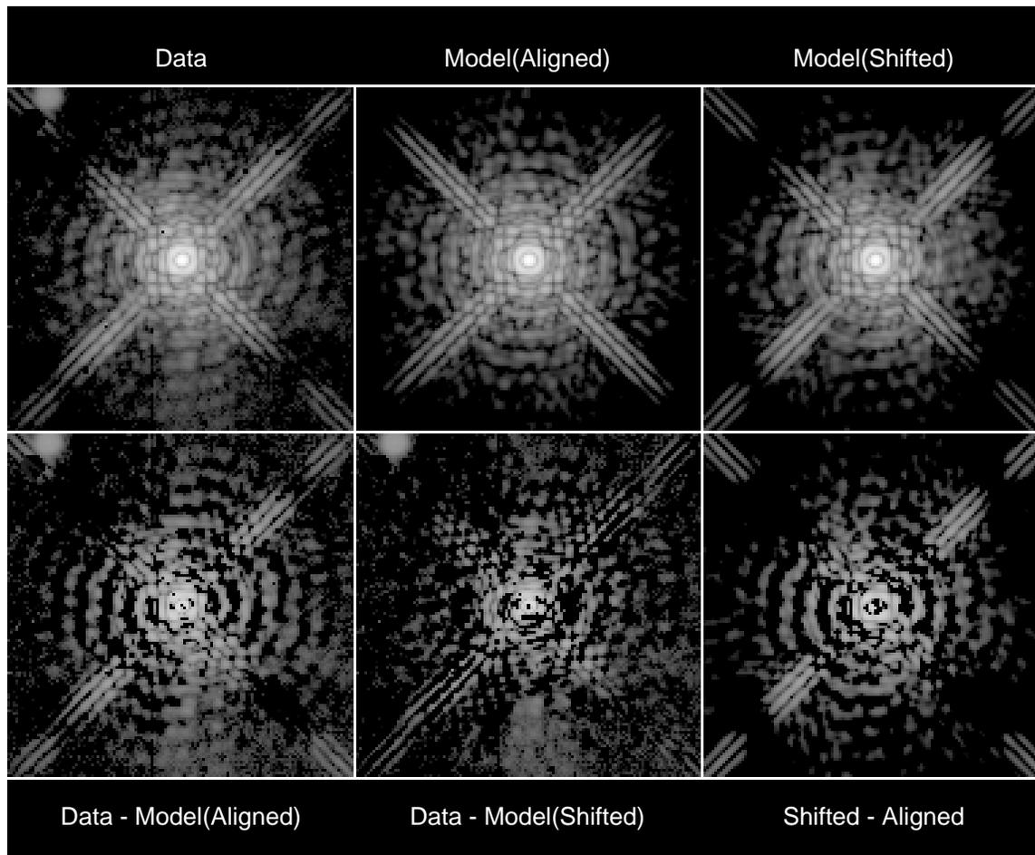
Figure 5. Results of Gerchberg-Saxton phase retrieval on a F222M NICMOS 2 PSF from the SNAP program. On the left is the observed PSF. The retrieved pupil amplitude after one iteration of the algorithm is shown in the middle. Note the elliptical central obscuration. After twenty iterations, the spiders are better defined.
