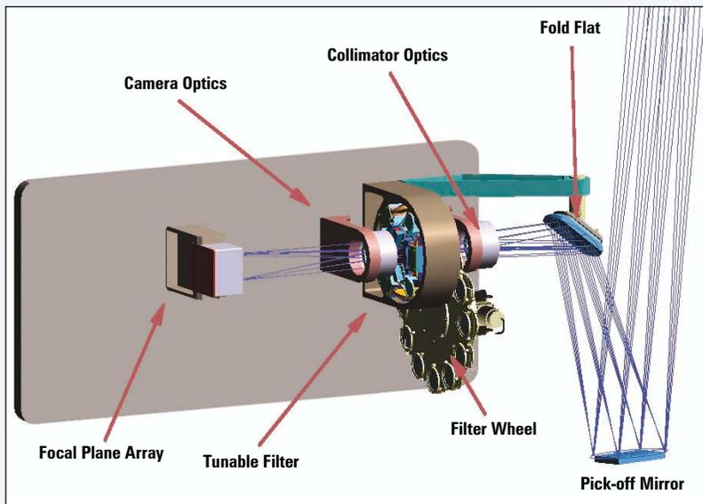
**Figure 2.** One of the tunable filter imaging models of the selected NIRCam design. The design has a total of four imaging modules: two tunable filter modules and two identical broad- and intermediate-band imaging modules.
