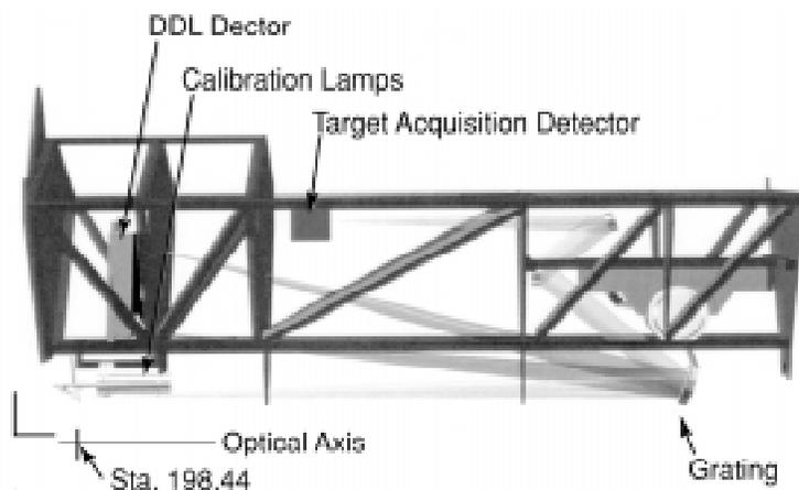
Figure 1: Schematic of the COS primary channel (as proposed). Light is received from the *HST* OTA through a 2-arcsecond round aperture, is dispersed by a concave diffraction grating, and finally is recorded on a curved double delay-line MCP detector adapted from the *FUSE* mission.
