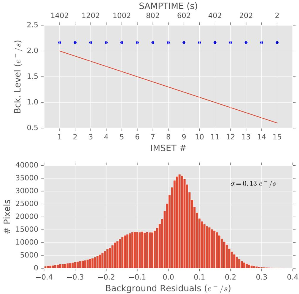
Fig. 3.—: **Significant background variation.** Same as Figure 2 but with a HeI background that varies significantly more ( $0.5e^-/s$  at the beginning of the exposure (IMSET 15) and rises to  $2e^-/s$ ). The fit once again assumes a constant background but the derived value is now incorrect ( $2.1e^-/s$  versus  $2e^-/s$ ) and the resulting background is highly non-gaussian (Bottom Panel). The standard deviation of the residuals is  $0.13e^-/s$ .
