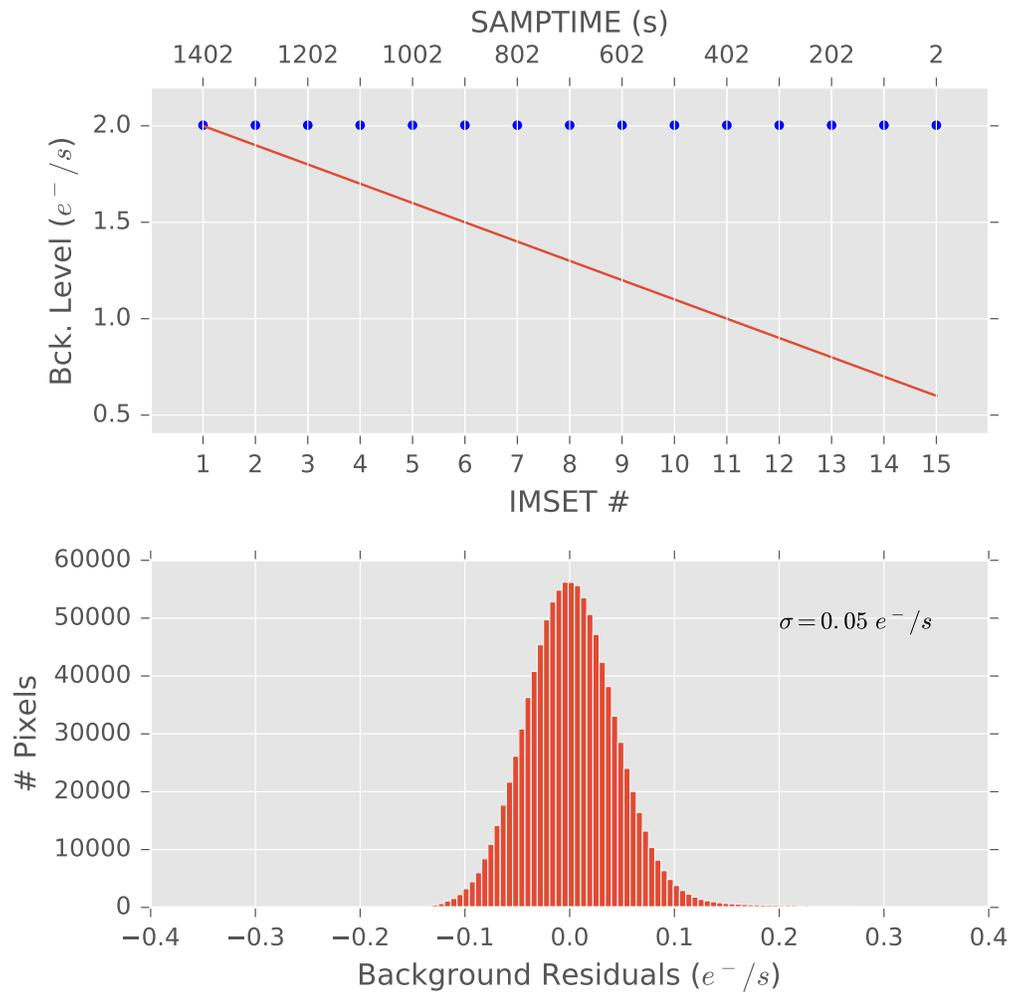
Fig. 4.—: **Significant background variation, "Last minus First" reduction.** Same simulated dataset as Figure 3 but now processing without up-the-ramp fitting. The estimated background level is now correct and the residuals are gaussian with a standard deviation of  $0.05e^-/s$ .
