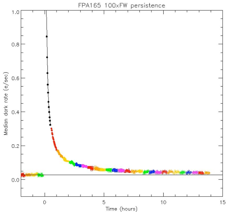
Figure 2: Background signal level measured at DCL, after illuminating the detector to signals of 100 times full-well.
