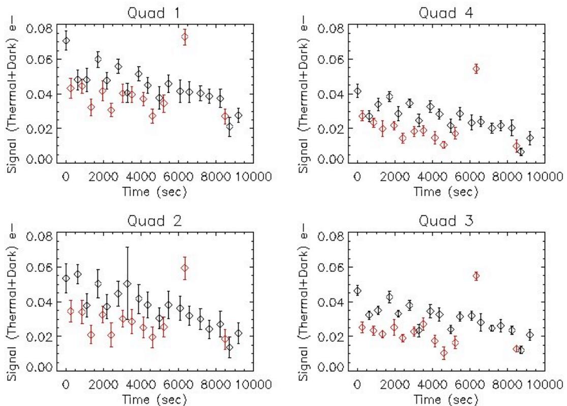
Figure 1: Median measured values of the dark current and background in the IR channel versus elapsed time of the test. Black points are signal rates in dark current files, while red points are those for filtered files, where each red point represents a different filter. Data were obtained moving from blue to red filters, so these plots can also be interpreted as being plotted versus increasing wavelength.
