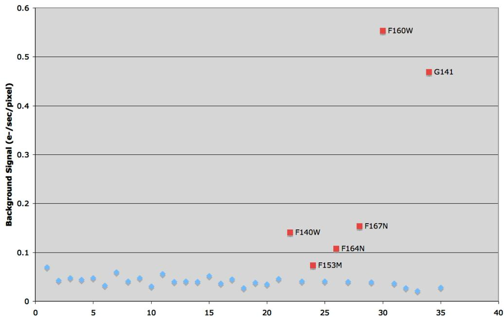
Figure 3: Expanded view of quadrant 1 in Figure 1. Filters where the thermal emission signal dominates are marked in red.
