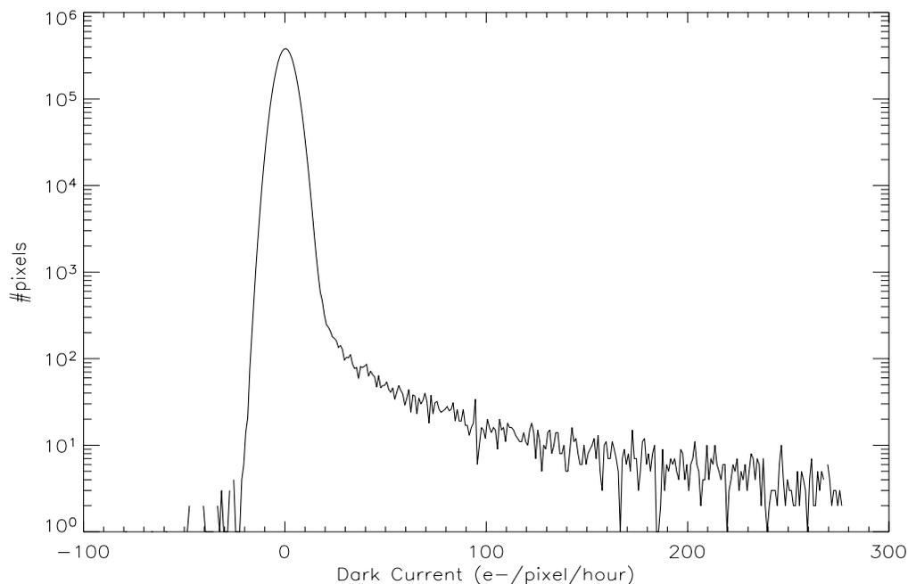
**Figure 2:** Histogram of dark current rates for the science pixels in Amp A in the unbinned 3000-second dark current file.
