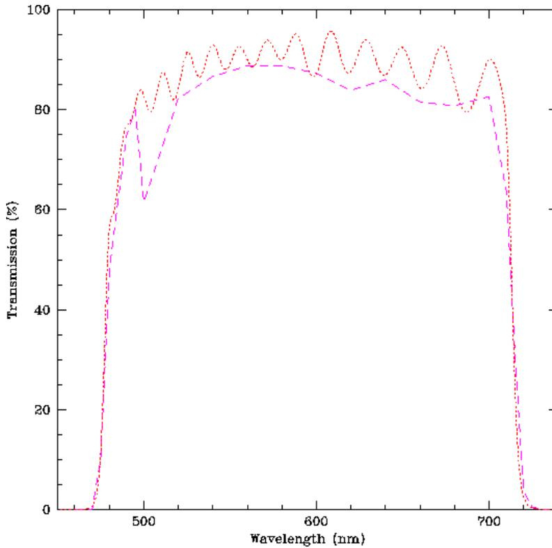
**Figure 11: Comparison between the expected (dotted line) and measured (dashed line) transmission profiles of the F606W filter.**
