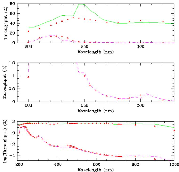
**Figure 4: Measured and predicted throughputs for the F218W filter. The green solid line gives the measured system throughput (i.e. with no filter in the SOFA), the magenta dashed line plots the filter data and the red triangles mark the predicted values.**
