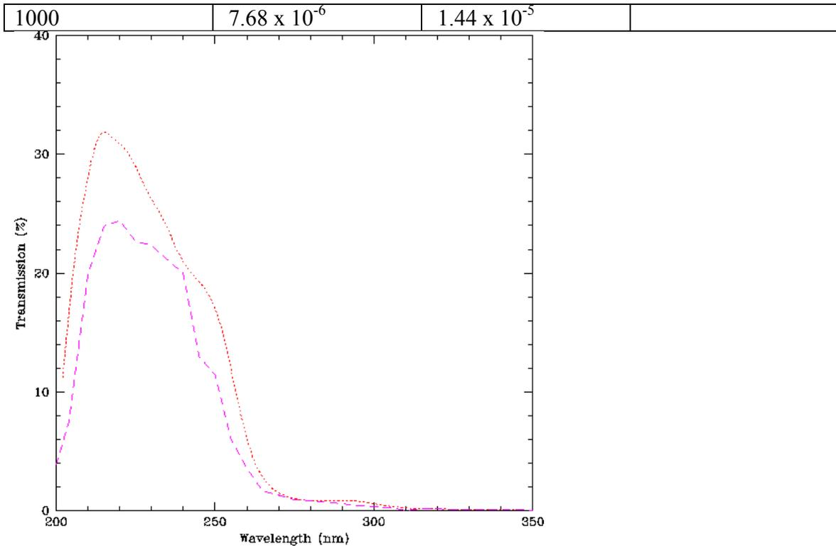
**Figure 7: Filter transmission for F225W - as in Figure 4, the dashed line plots our measurements and the dotted line outlines the pre-installation data.**
