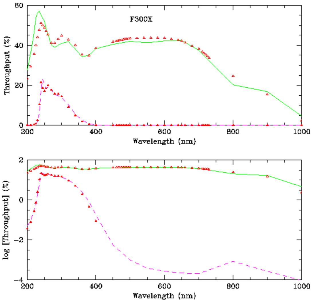
**Figure 8: Throughput measurements for F300X.** As in Figures 3 and 5, the filter throughput data are plotted as a dashed line, while the system throughput (CLEAR) is shown as a solid line. Solid and open triangles mark the predicted throughput values for the system and filter, respectively.
