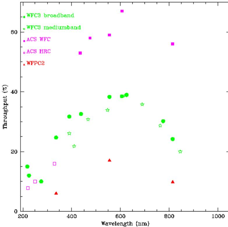
**Figure 3: Comparison between the measured throughput of WFC3, ACS and WFPC2.** The WFC3 data are taken from Table 1; ACS WFC data are for the F450W, F500, F555W, F606W and F814W filters; ACS HRC data are for F220W, F250W and F350W filters; and WFPC2 data are for the F336W, F555W and F814W filters.
