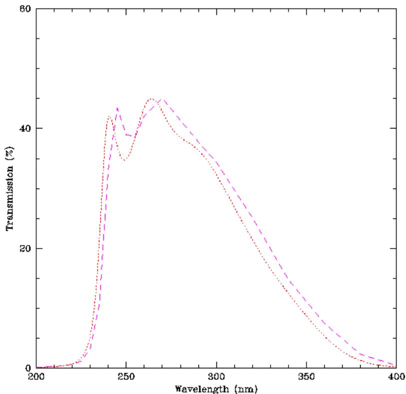
**Figure 9: Transmission profile for f300X filter. As in previous figures, the dashed line plots the empirical results, and the dotted line the expected profile, based on pre-installation measurement.**
