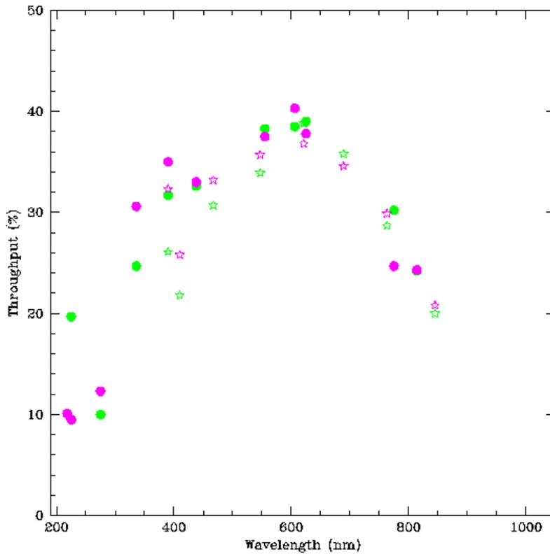
**Figure 2: Broad- and medium-band filter throughputs.** The predicted values are shown in magenta, the measured values in green, with broadband filters plotted as filled points and medium-band filters as stars. No quantum effect corrections have been made to either predicted or observed values.
