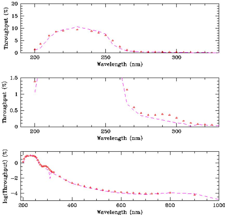
Figure 6: Throughput measurements for F225W. The dashed line marks empirical measurements of the filter throughput, while the open triangles plot the expected values.
