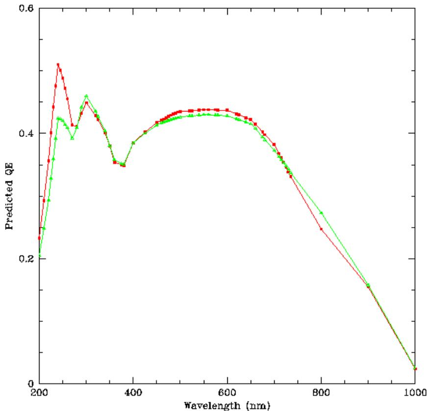
**Figure 1** Expected throughput for the two Marconi CCDs installed in the UVIS camera. Chip 1 (CCD c178) is plotted in green; chip 2 (CCD c018) in red. These data are derived using the GSFC Detector Characterization Laboratory (DCL) measurements of CCD quantum efficiency and the predicted throughput of the WFC3 UVIS optical components (excluding photometric or spectroscopic filters).
