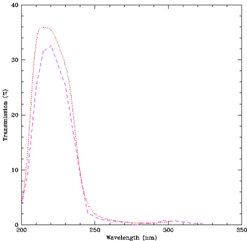
**Figure 5: Transmission curve of the F218W filter. The dashed line shows the values deduced from our measurements, while the dotted line plots measurements of the transmission before installation in the SOFA**
