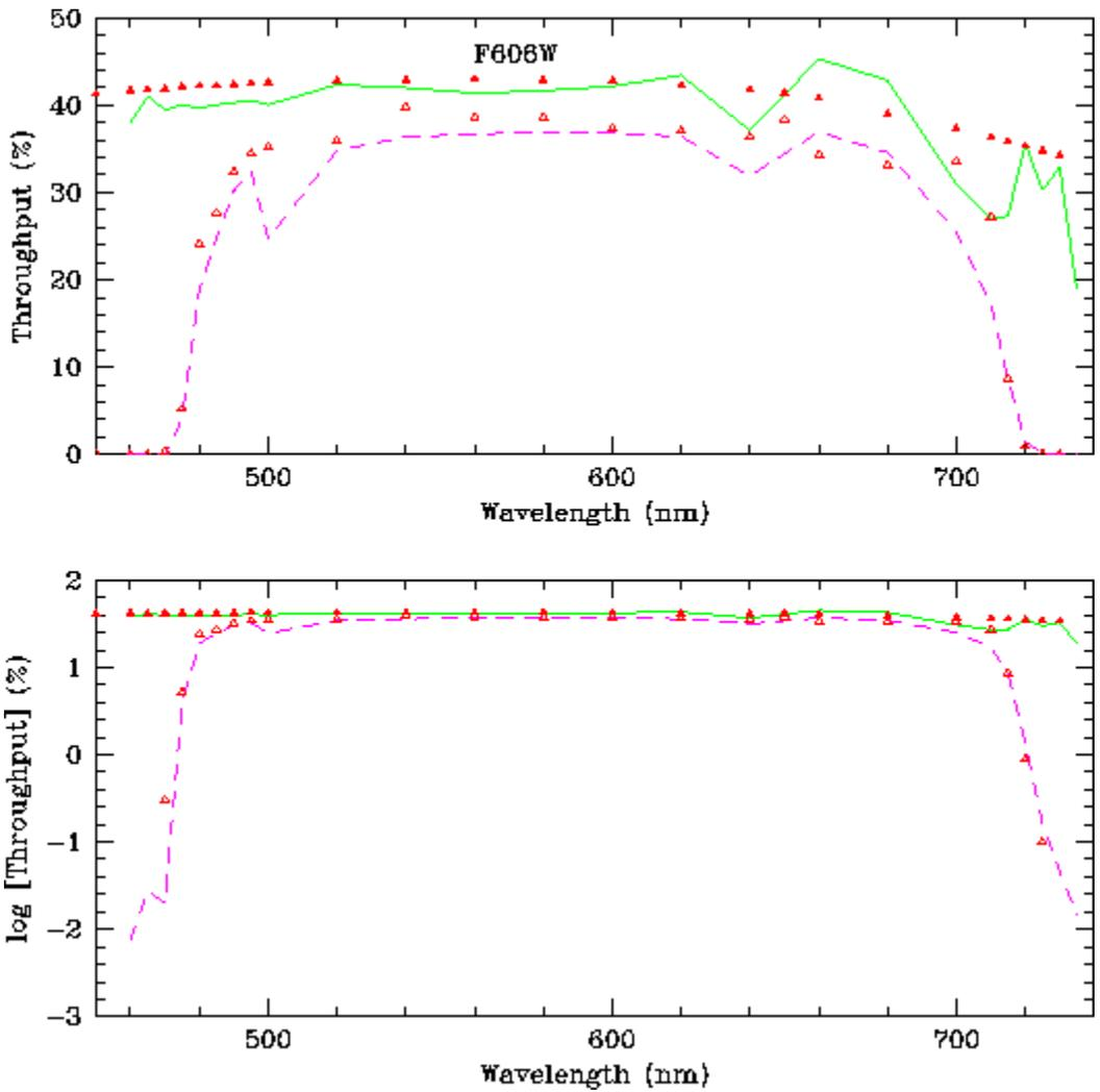
Figure 10: Throughput measurements for the F606W filter. As in previous figures, filter throughput data are plotted as a dashed line, while the system throughput (CLEAR) is shown as a solid line. Solid and open triangles mark the predicted throughput values for the system and filter, respectively.
