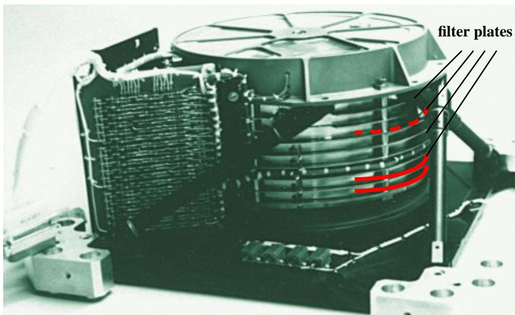
**Figure 4: WFPC1 Selectable Optical Filter Assembly (SOFA).**
