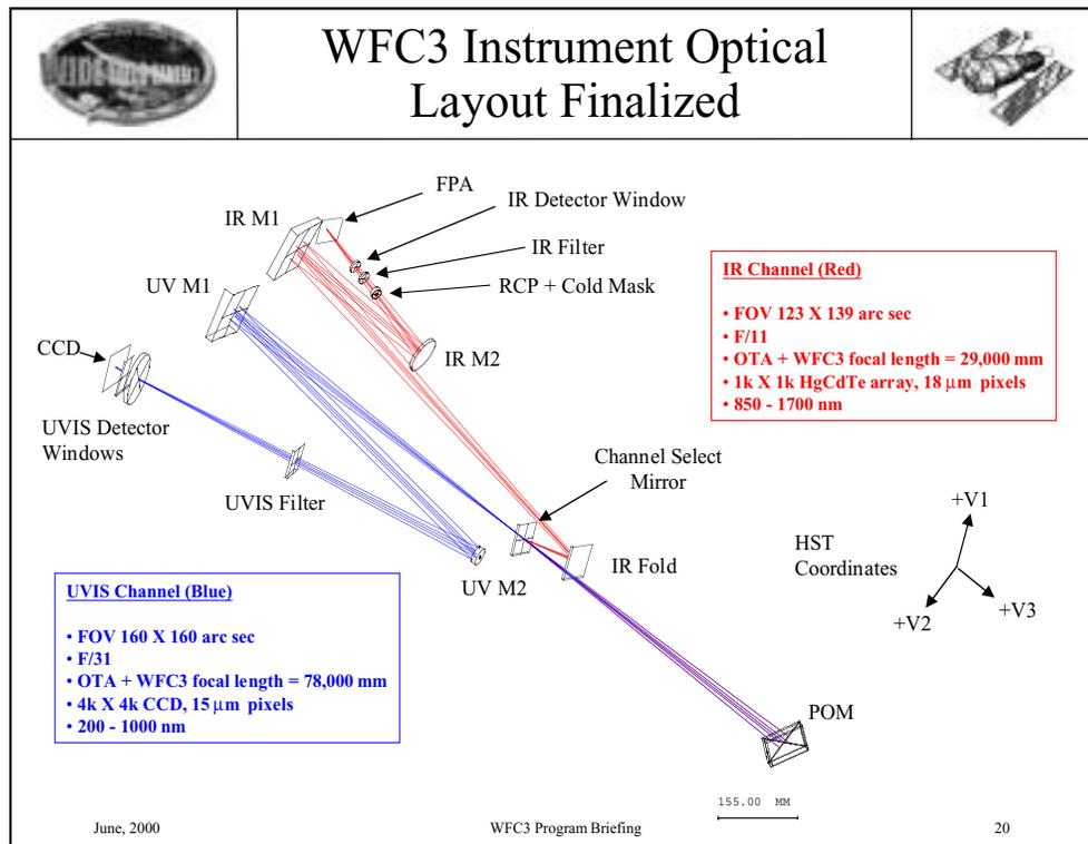
**Figure 3: WFC3 UVIS and IR Optical Design.**
