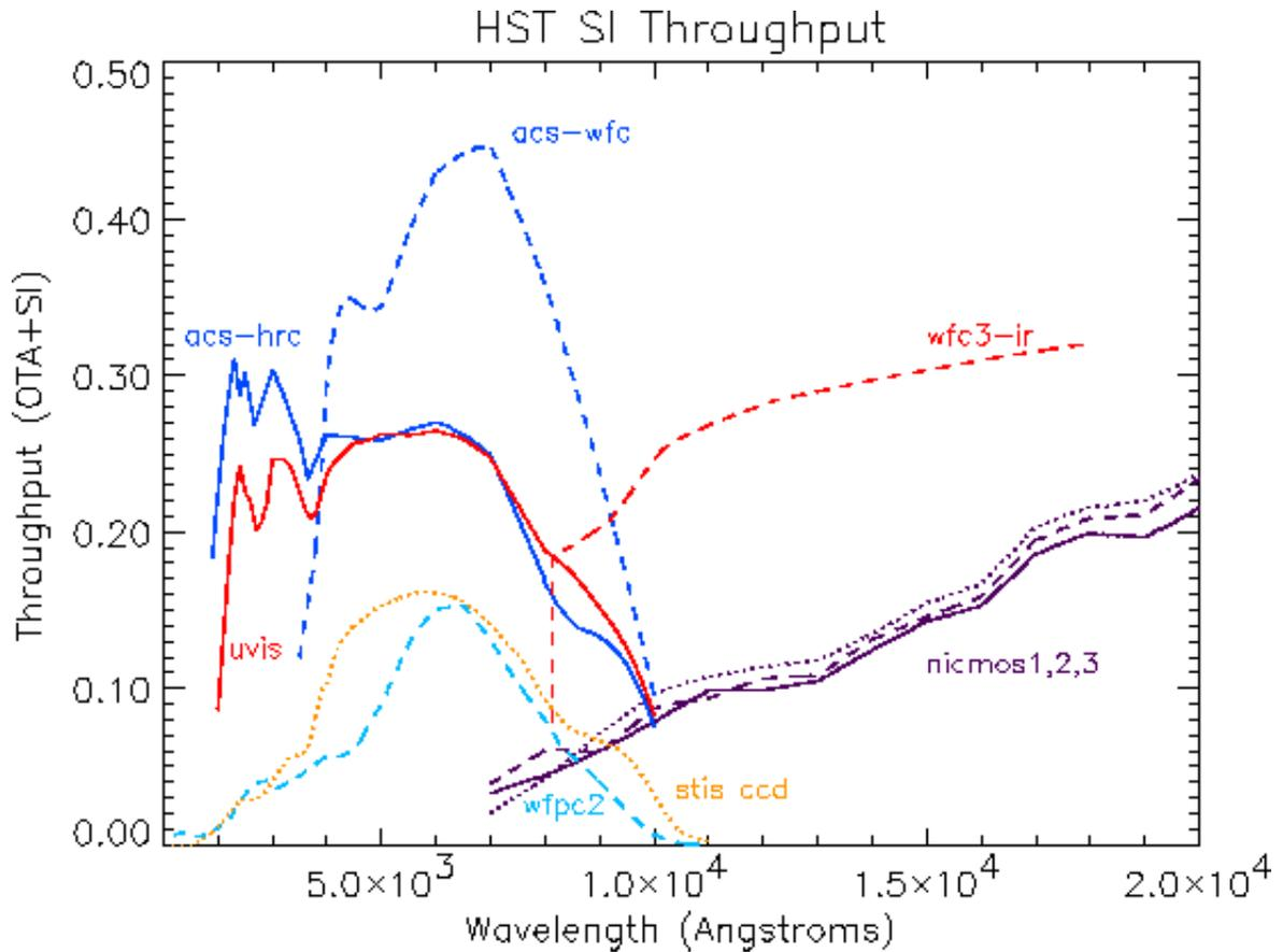
**Figure 1: HST Instrument Throughput Curves.** The WFC3 IR curve is from a Hawaii device, the WFC3 UVIS curve is a Lesser-coated SiTe CCD. WFC3 values are approximate.
