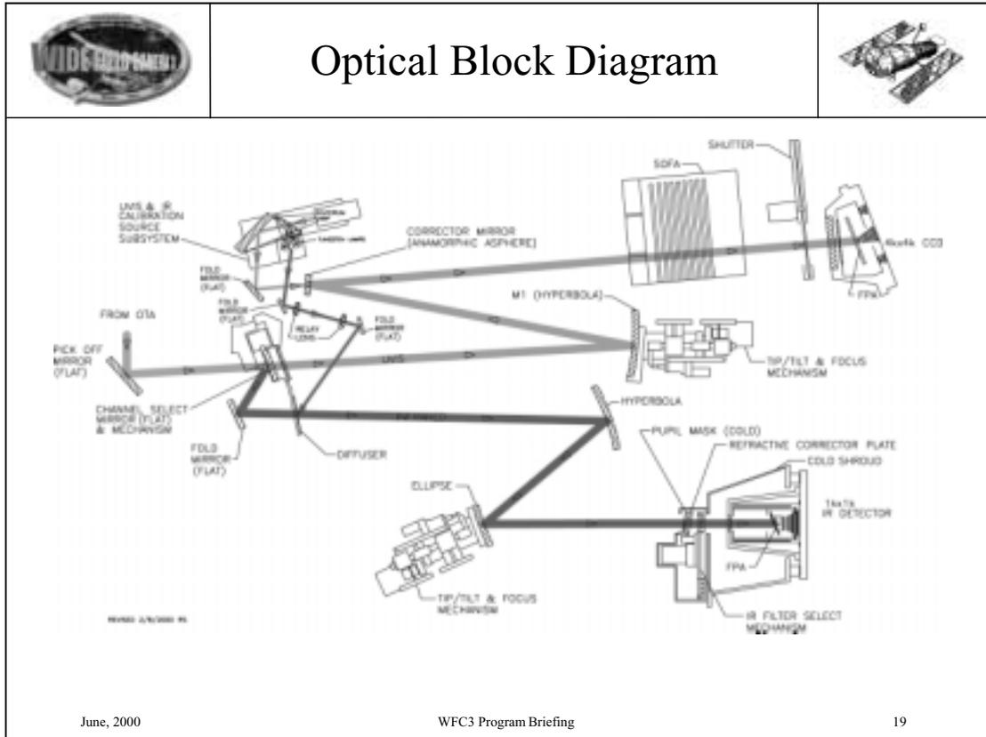
Figure 2: WFC3 UVIS and IR Channel Block Diagram.
