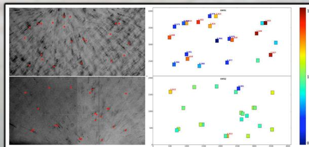
**Figure 4** – F218W flat field (left) and photometric residuals (right) computed from stepping a star across the detector. Dark portions of the fishscale pattern represent regions of lower QE in the flat, and these produce photometry which is systematically too faint using the pipeline flats.
