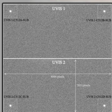
**Figure 1** – The to-scale locations of the four corner 512 pixel subarrays on the WFC3 two-chip mosaic. From Kalirai, et al. 2010.
