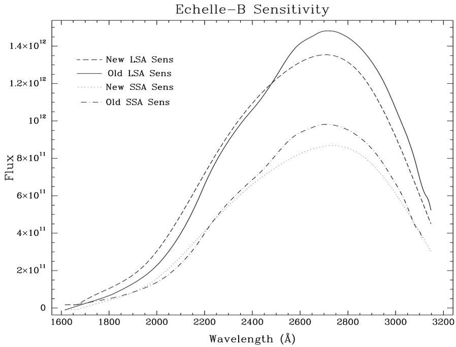
**Figure 4:** The previous sensitivity functions are plotted with the corrected curves, illustrating the extent of the change required to match the Echelle-B data with the reference spectrum of  $\mu$  Col.
