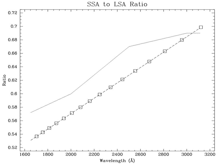
**Figure 3:** The SSA/LSA ratio is plotted for each of the POST-COSTAR sensitivity functions (e5v0936oz.r3h=dotted line, e4e13583z.r3h=box+dashed line). We adopt the later for our determination of the SSA sensitivity.
