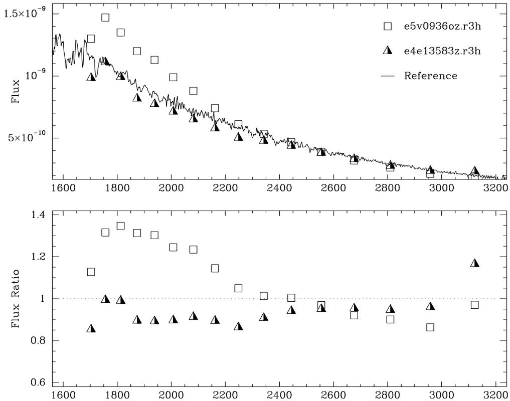
**Figure 2:** The reference flux for  $\mu$  Col is plotted with the calculated values from Echelle-B. *a)* The Cycle 4 observations derived using the recommended sensitivity function (boxes) and the previous sensitivity function (triangles) are overplotted on the reference spectrum. *b)* The flux ratio shows the extent of the deviations for each file.
