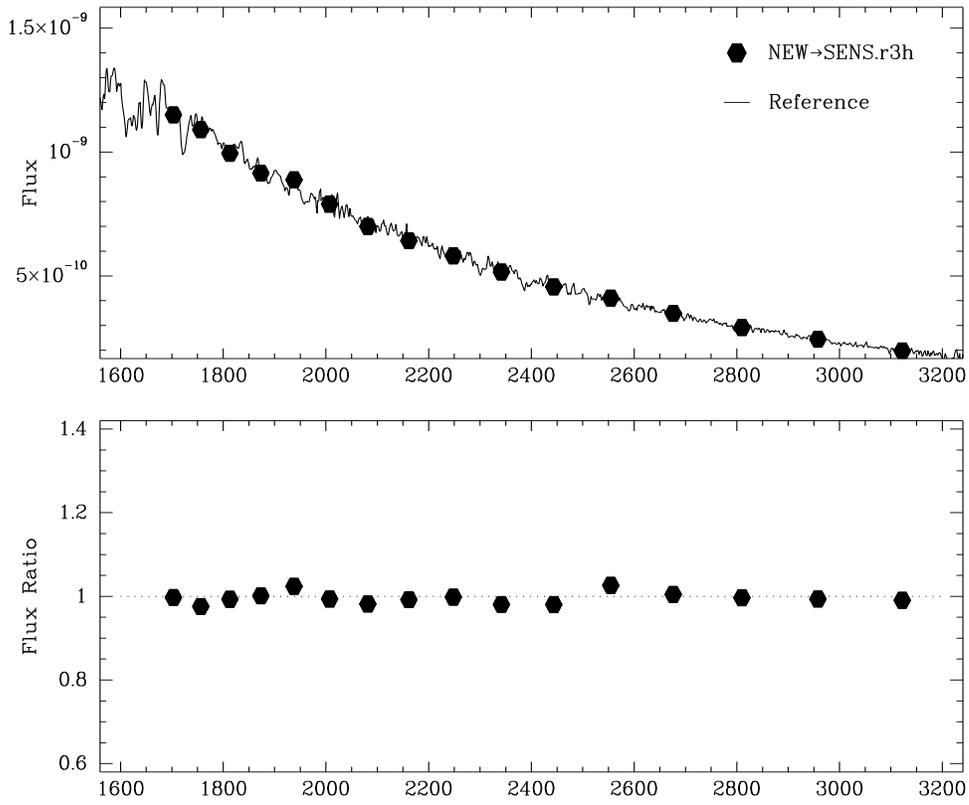
**Figure 5:** *a)* The reference flux for  $\mu$  Col is plotted with the recalibrated values from Echelle-B, using the new sensitivity function. *b)* The flux ratio improves dramatically, from a standard deviation of 17% down to only 1.4%
