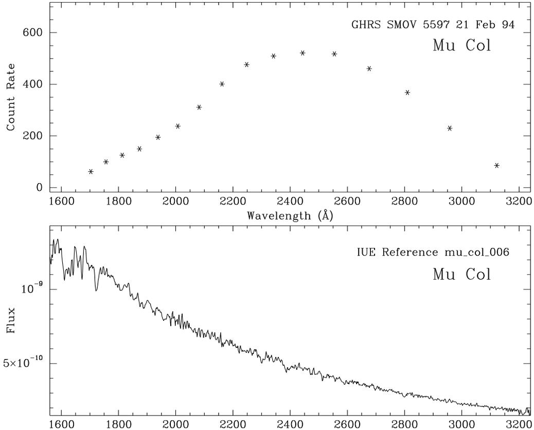
**Figure 1:** Observed spectra  $C_\lambda$  of standard star  $\mu$  Col with GHRIS Echelle-B compared to its reference spectrum  $F_\lambda$  taken with the IUE.
