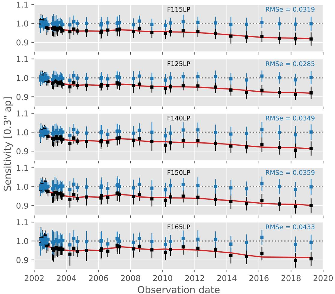
**Figure 3:** Initial sensitivity measurements for each filter in this study. Black boxes are the mean and standard deviation of the sensitivity before any TDS correction. The red line is the extracted TDS. Blue boxes are the sensitivity after applying TDS correction.
