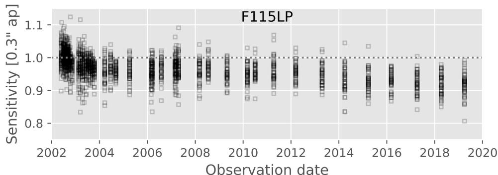
**Figure 2:** Sensitivity measurements as a function of time for the F115LP filter. Each box represents a measurement for an individual star. The number of boxes per date varies, as some stars may not have valid data on a given date.
