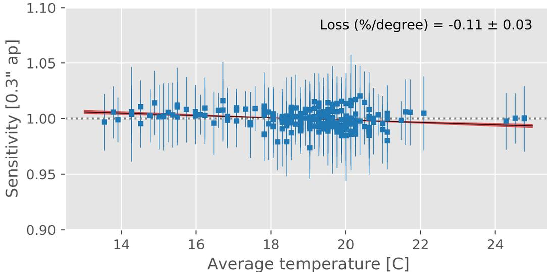
**Figure 7:** Sensitivity with respect to detector temperature at time of observation. These points include the TDS correction. All filters are included in this plot.
