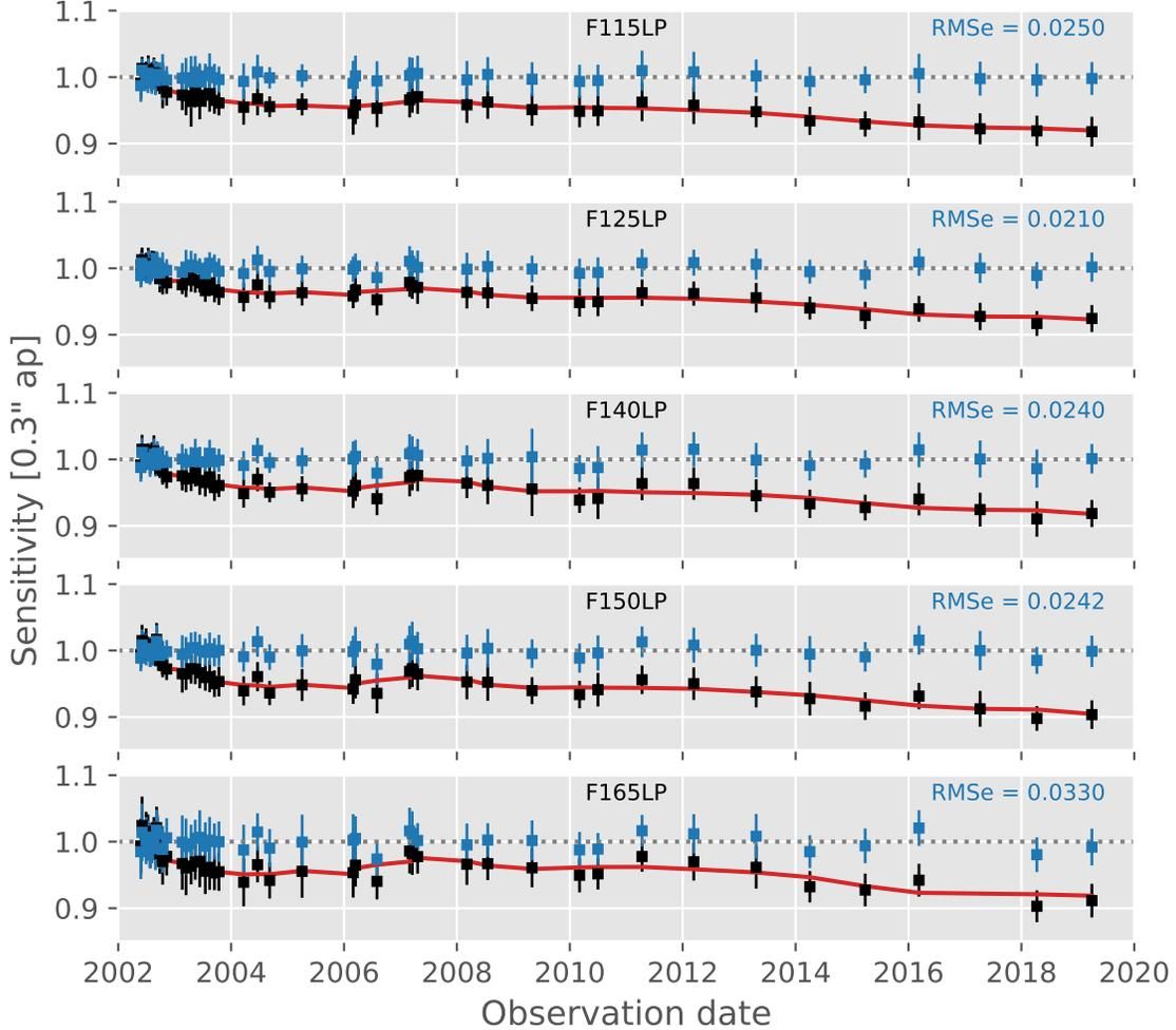
**Figure 6:** Final sensitivity measurements. Black boxes are the mean and standard deviation of the sensitivity before any TDS correction. The red line is the extracted TDS. Blue boxes are the sensitivity after applying TDS correction.
