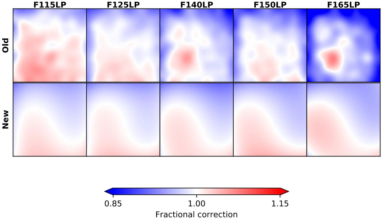
**Figure 5:** The old and new L-flat frames. The colors indicate the L-flat contribution to the fractional correction that is applied when an image is divided by the LP-flat. All images are presented with the same stretch.
