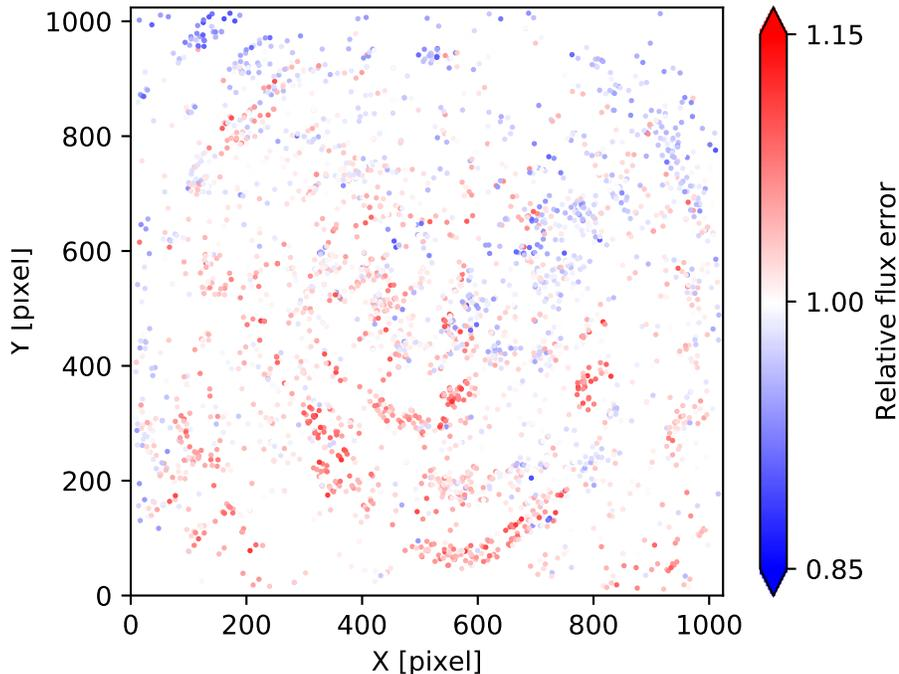
**Figure 4:** Relative flux error as a function of position on the detector. Red points are measurements that were higher than the mean, blue were lower.
