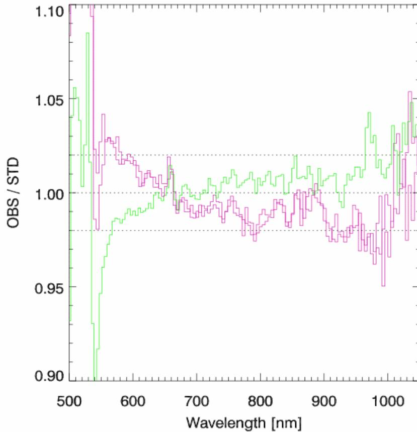
**Figure 4:** The aXe extracted spectra of the standard star GD153, shown as the ratio of the observed flux over the model spectrum versus wavelength. Observations obtained on different CCDs are color-coded, as indicated in Figure 3.
