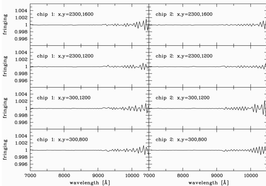
**Figure 9:** The effect of fringing determined by dividing the spectrum without fringe amplitudes applied with the spectrum to which calculated fringe amplitudes were applied to the CCD pixels before the extraction. The panels address various point-like objects at different positions across both CCD chips.
