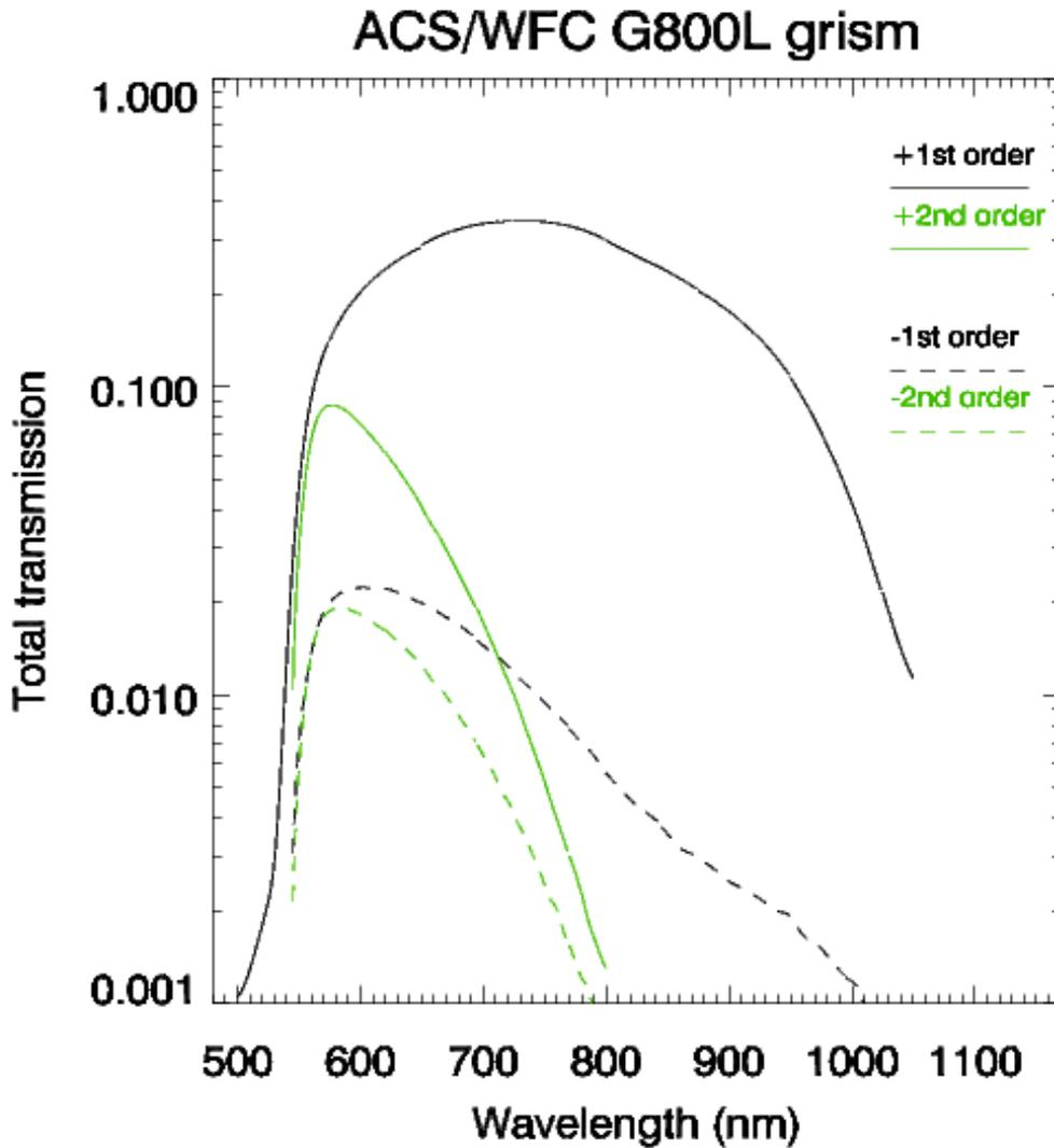
**Figure 5:** Total throughput of the +1<sup>st</sup>, +2<sup>nd</sup>, -1<sup>st</sup>, and -2<sup>nd</sup> orders of the G800L grism in the WFC, derived from the sensitivity curves of this report.
