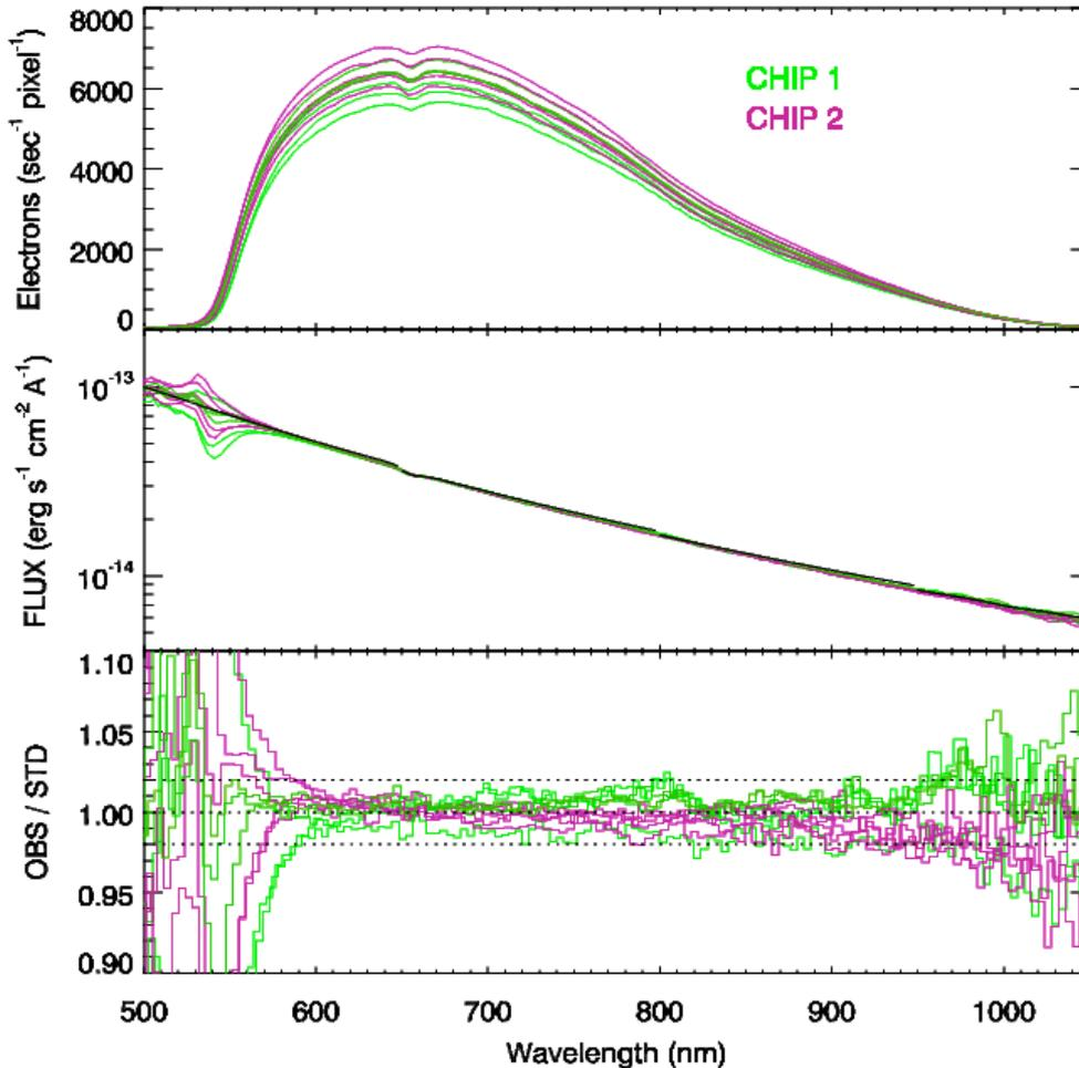
**Figure 3:** The aXe extracted 1-dimensional spectra of the standard star G191B2B in units of electrons per second per pixel, fully calibrated flux units and the ratio of the observed flux over the model spectrum versus wavelength (from top to bottom). Observations obtained on different CCDs are color-coded as indicated in the upper panel.
