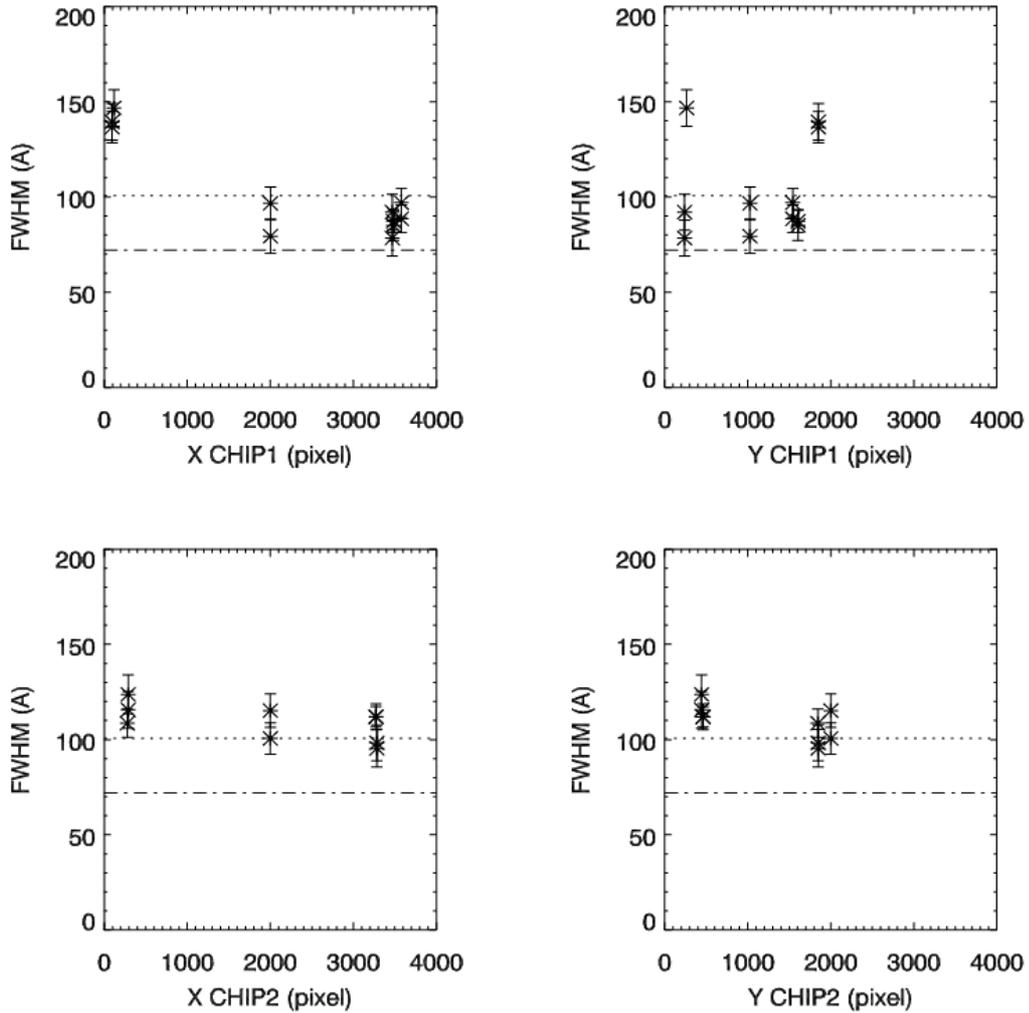
**Figure 8:** Spectral resolving power (FWHM in Å) as determined from the H $\alpha$  line of the standard star G191B2B for 20 different exposures at various spatial positions. The dotted line shows the median value. The long dash-dotted line shows the expected spectral resolving power if only the HST/ACS point spread function is taken into account (see text for details).
