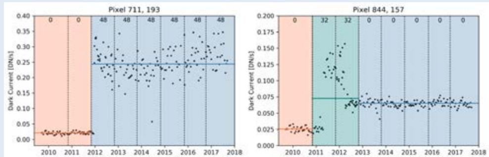
Temporal behavior of two of the IR channel pixels. Pixel 711, 193 (left panel) remained cold and stable for the first three years of operation and then became warm and stable. Pixel 844,157 was cold and stable the first two years of operation, was unstable from 2011 to 2013, and has been cold and stable for the past 5 years.
