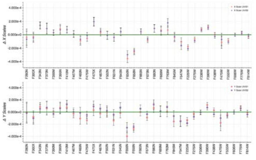
Difference along the X (top panel) and the Y (bottom panel) axis between the plate scale values for every UVIS filter and the reference filter F606W, for both Chip1 (in orange) and Chip2 (in purple).
