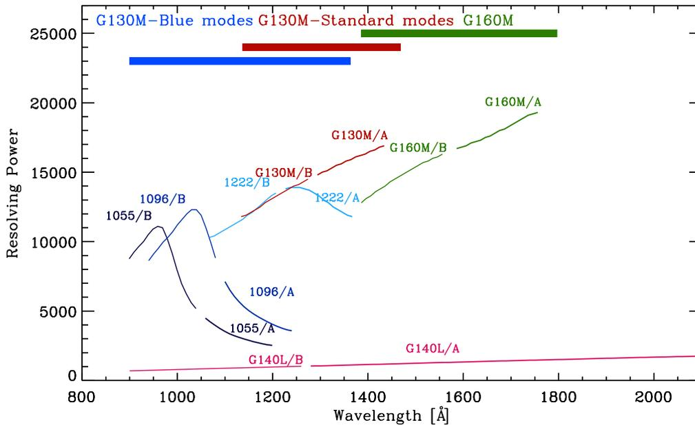
COS/FUV resolution as function of wavelength for Cycle 25+
