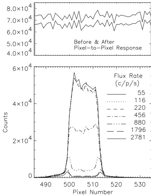
Figure 3. Showing the detector response to an image that is many times brighter than the local dynamic range. Localized gain sag within the MCP at the location of the image causes a temporary loss in counting efficiency leaving the rest of the detector unaffected. This test also demonstrates the safety and robustness of the MAMA detector to bright localized sources for brief periods of time.
